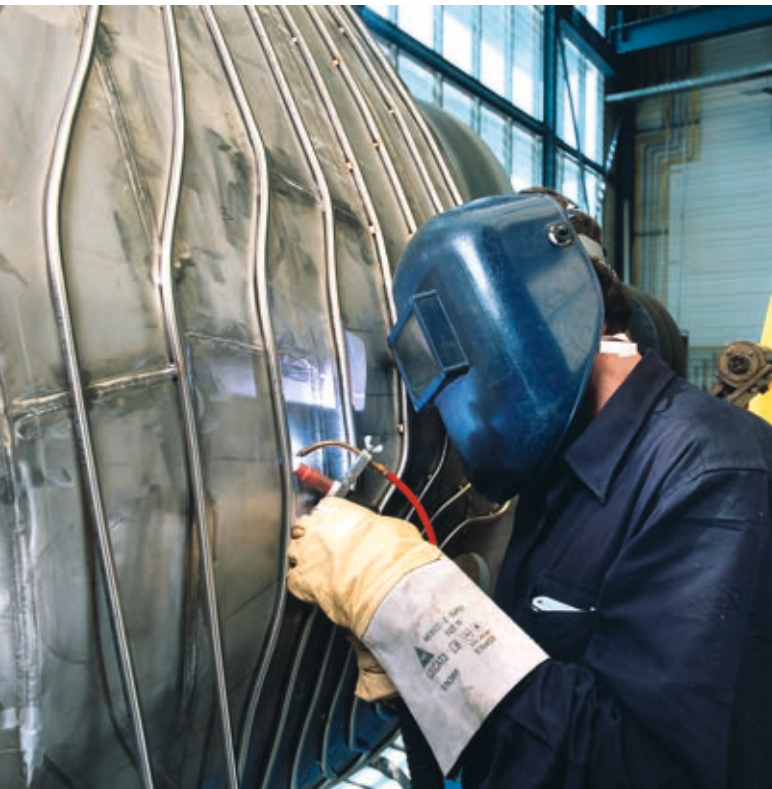
Welding the Wendelstein 7-X plasma vessel
