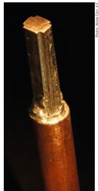
HTS CrossConductor with additional copper cladding
