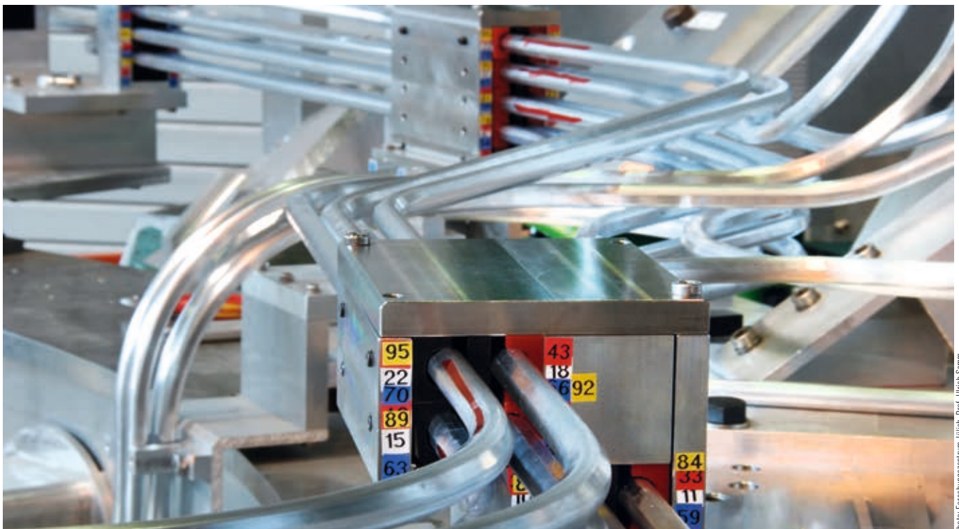
Geometric check of shaped superconductors
