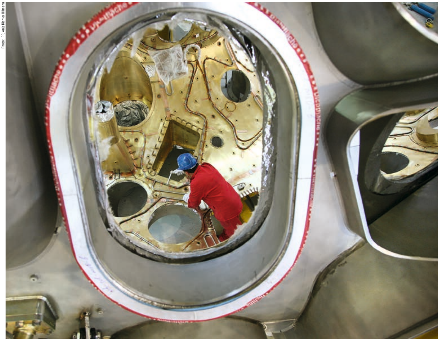
Assembly of the thermal insulation for the outer vessel (brass shields)
