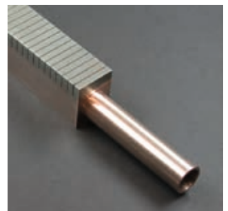
Mock-up of a plasma-facing component with a heat sink made of tungsten particle-reinforced copper composite material
