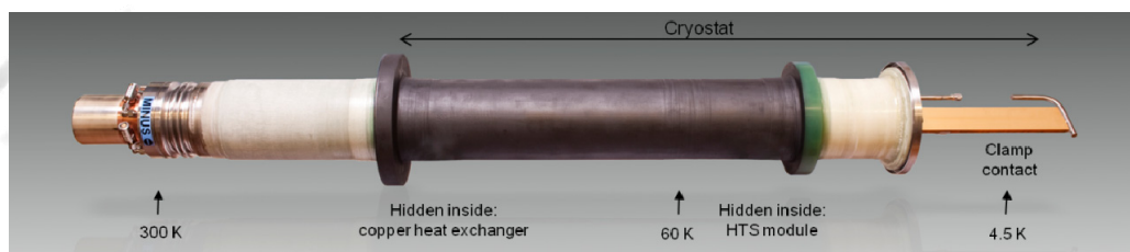
Figure 1: Photograph of the W7-X current lead prototype developed at KIT and IPP. During operation, the left side is at room temperature, while the right side is connected to the superconducting coils. The heat exchanger is based on a development from CERN.
