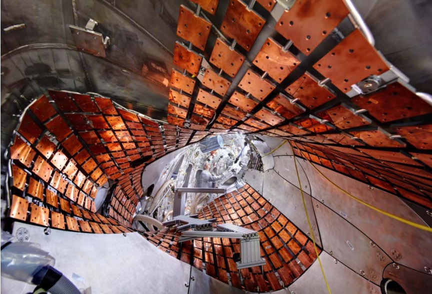
View into the plasma vessel before the first operation phase. In the mean time, precisely fitting graphite tiles have been mounted over these wall protection elements made of copper-chromium-zircon.
