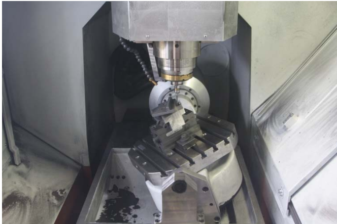
Machining of a graphite tile on the five axis milling machine
