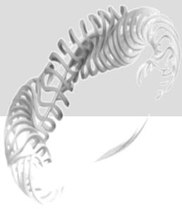
Since Wendelstein 7-X is designed for steady-state operation, its divertor has been designed to withstand quasi-continuous heat fluxes of up to  $10 \text{ MW/m}^2$  and a maximum total load of  $10 \text{ MW}$  is to be handled for about 30 minutes. For safe operation of the divertor and to learn how to reduce impurity content and power loads, diagnostics have been installed to measure important plasma quantities.
