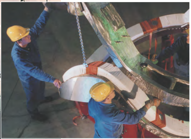
Magnet coils for Wendelstein 7-X
