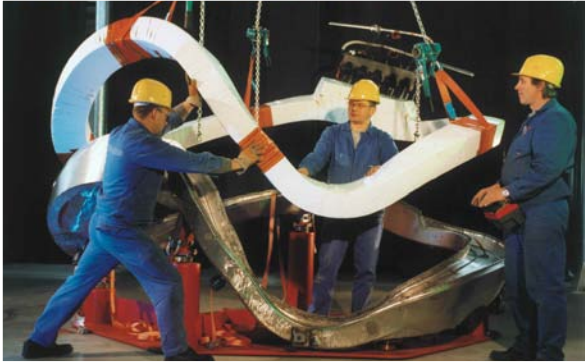
Superconducting magnet coil during production
