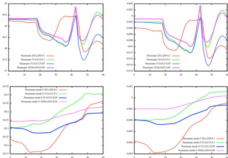
**FIGURE:** Long time evolution of electric energy (left) and relative mass error (right) for Neumann (top) and Neumann mode 0 (bottom) boundary conditions, with different discretizations ( $N_r \times N_\theta \Delta t$  on legend).
