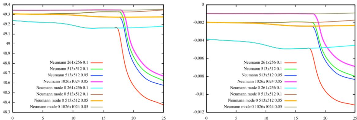
**FIGURE:** Time evolution of electric energy (left) and relative mass error (right) for Neumann and Neumann mode 0 boundary conditions, with different discretizations ( $N_r \times N_\theta \Delta t$  on legend).
