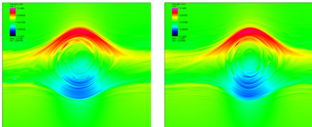
FIGURE:  $f(1000, x, v) - f_0(x, v)$ ,  $\Delta t = 0.05$ . Cubic splines, with  $N_x = N_v = 4096$  on CPU (left) and Lagrange interpolation of degree 17  $N_x = N_v = 2048$  on GPU double precision (right).
