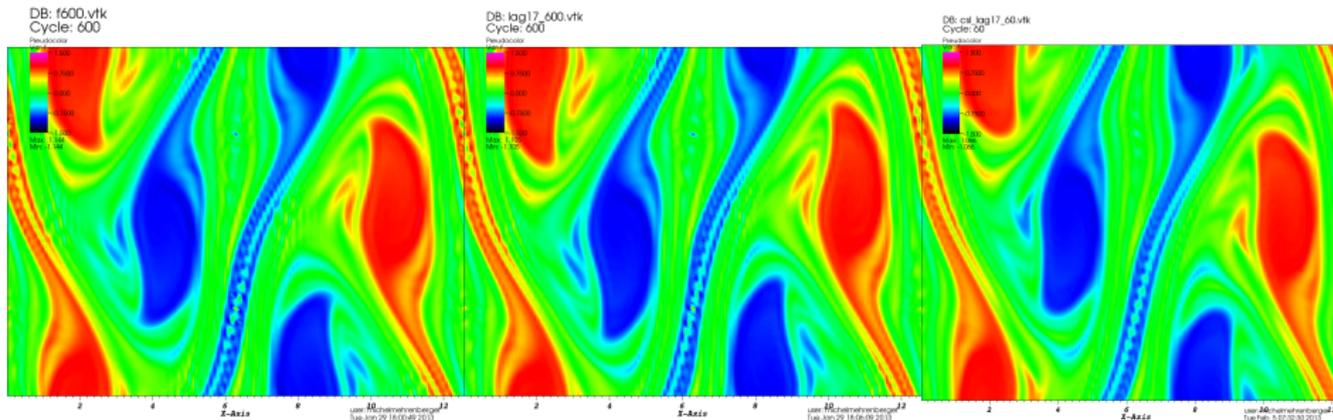
**FIGURE:** Distribution function at time  $T = 60$ ,  $\Delta t = 0.1$ ,  $N = 128$  Advective 2D cubic splines (left), advective 2D FD(17) (middle), conservative 2D FD(17) (right)
