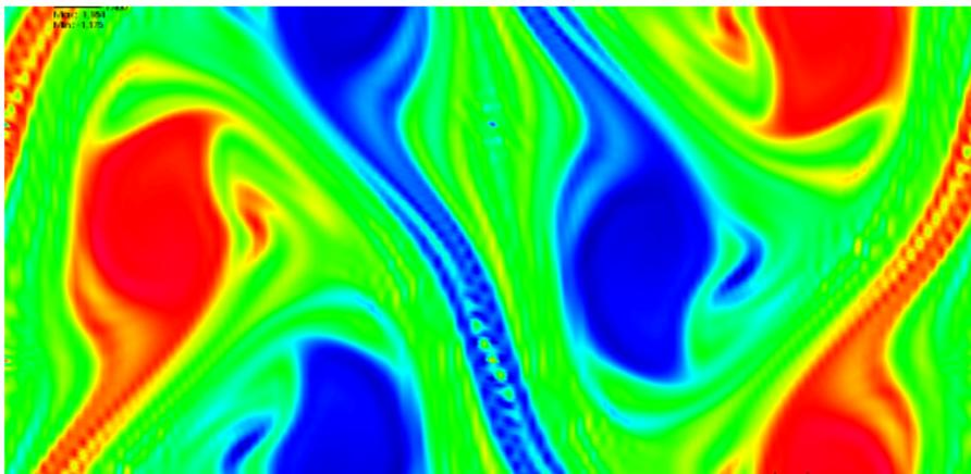
**FIGURE:** Distribution function at time  $T = 60$ ,  $\Delta t = 0.1$ ,  $N = 128$  classical advective cubic splines,  $\alpha = 10^{-1}$
