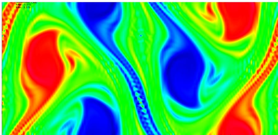
**FIGURE:** Distribution function at time  $T = 60$ ,  $\Delta t = 0.1$ ,  $N = 128$  classical advective cubic splines,  $\alpha = 10^{-6}$
