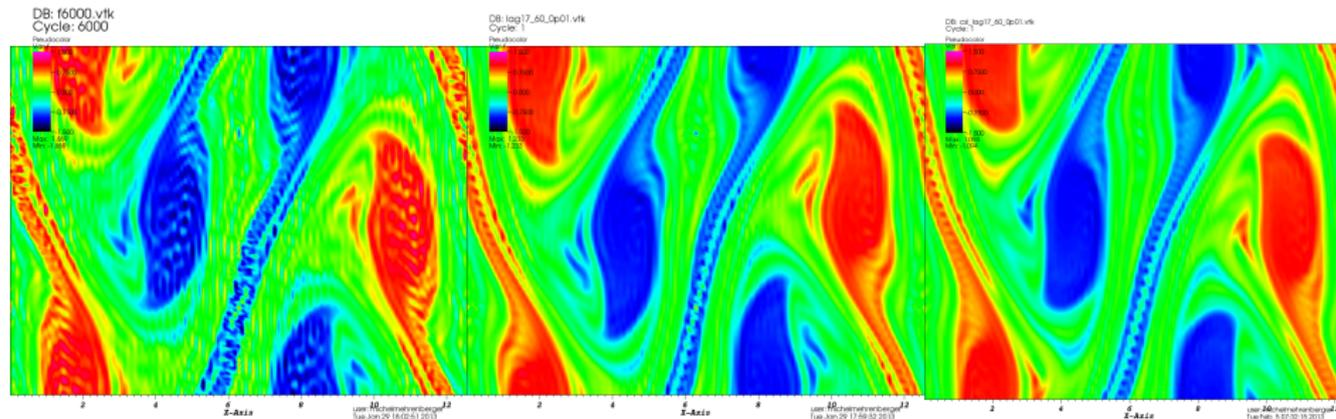
**FIGURE:** Distribution function at time  $T = 60$ ,  $\Delta t = 0.01$ ,  $N = 128$  Classical advective 2D cubic splines (left), advective 2D FD(17) (middle), conservative 2D FD(17) (right)
