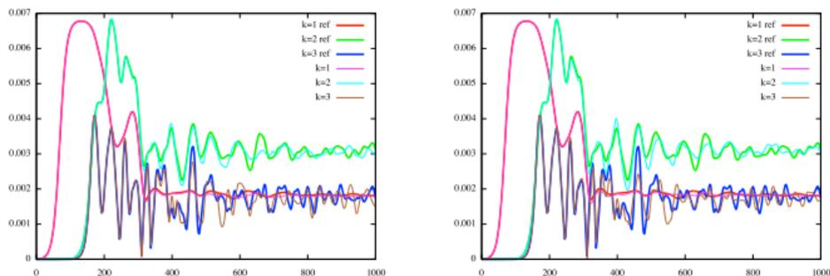
**FIGURE:** Absolute values of the first three Fourier modes of  $\rho$  vs time. Reference solution with LAG17  $N_x = N_v = 2048$  on GPU double precision (red, green and blue) compared to solution on uniform mesh in space (LAG17,  $N_x = 256$ ) and uniform refined mesh in velocity with  $N_v = 374$  ( $N_{\text{coarse}} = 64$ ,  $N_{\text{fine}} = 2048$ ,  $i_1 = 34$ ,  $i_2 = 44$ )
