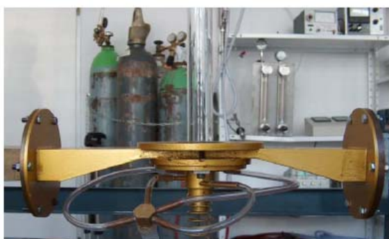
Fig. 1. Waveguide-based cylinder-type (nozzleless) MPS operated at atmospheric pressure and high gas flow rates. The inner diameter of the quartz cylinder is 26 mm.
