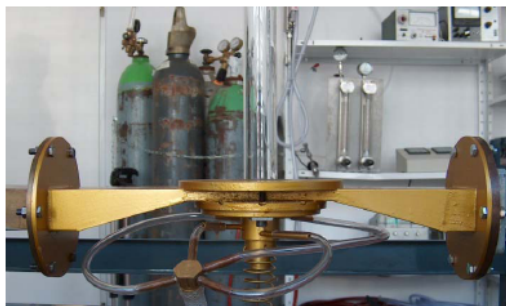
Fig. 1. Waveguide-based (nozzleless) MPG operated at atmospheric pressure at high gas flow rates. The inner diameter of the quartz cylinder is 26 mm.
