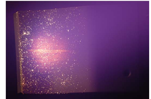
No damage in cycling up to 1600°C
