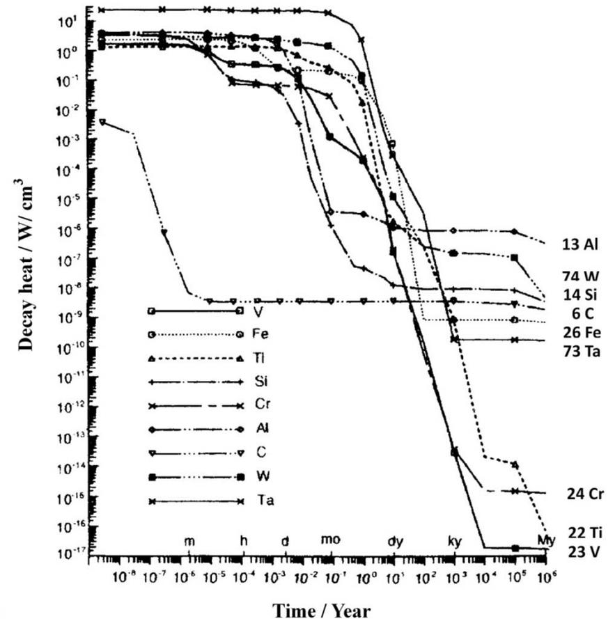
Induced radiation (left) and decay heat (right) of selected materials by typical neutron spectrum in fusion reactor.
