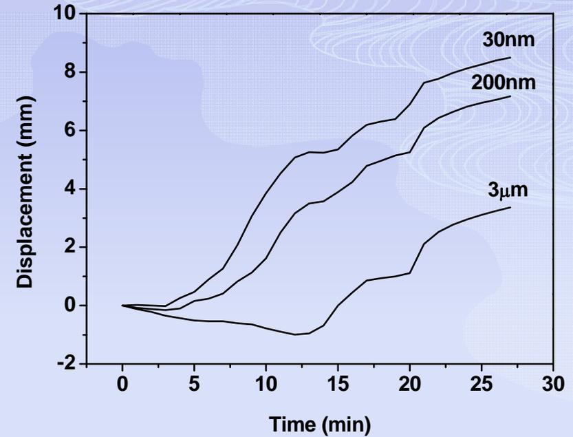
Green compact of tungsten is 20mm in diameter and about 6mm in thickness. Spark plasma sintering of samples is at 1700 °C under 50 MPa for 5 minutes. The finer tungsten powder is, the lower relative density of the sample is.
