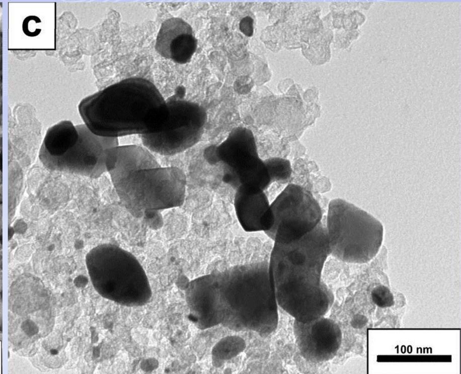
Transmission electron micrograph of TaC nanopowders prepared in Ar at 1400 °C
