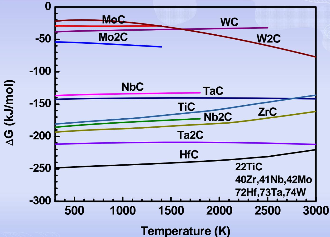
Tantalum carbide is stable near to titanium carbide. Bitantalum carbide is stable near to hafnium carbide. Atomic number of Tantalum only inferior to tungsten.
