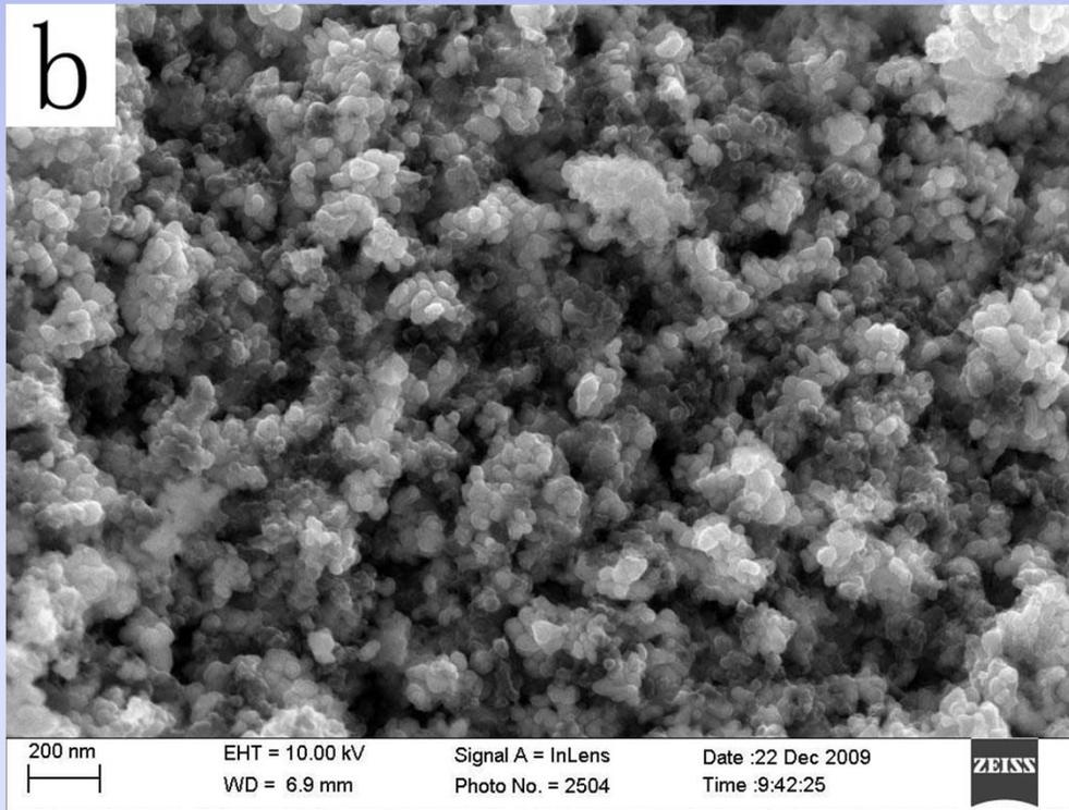
Scanning electron micrograph of TaC nanopowders eliminated free carbon
