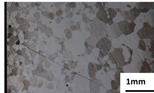
LM-images of cross-section after the three pulses
