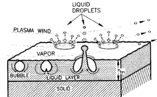
Fig. 4. Bubble growth, vaporization and loss by incident plasma wind.
