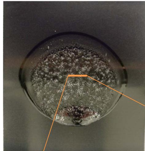
Melt ejection leads to loss of parts of the melt layer.
