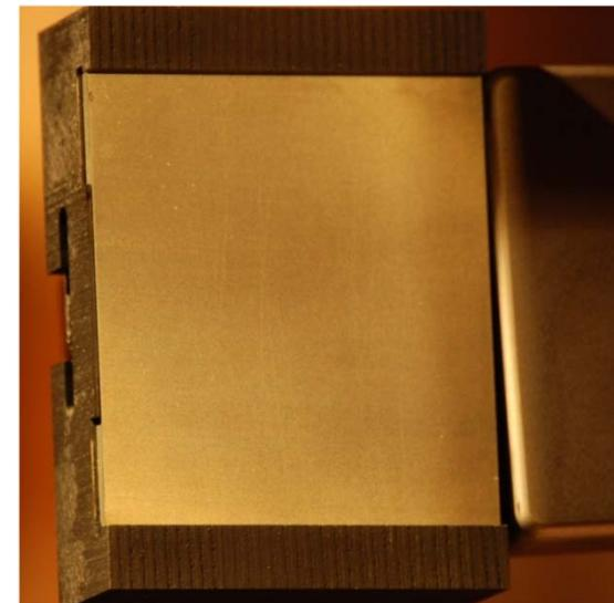
Sample surface  $\perp$  the beam axis
