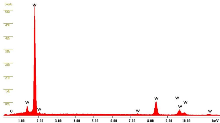
EDX for the deposited droplet
