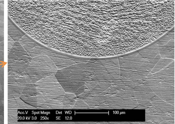
Droplets ejection under high heat flux loads
