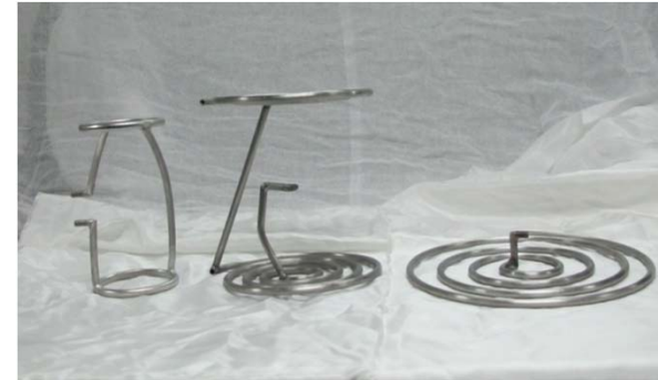
Three type HWP antennas; Movable antenna will be transferred to the center of plasma vessel; Bt is perpendicular to the circle of antenna.
