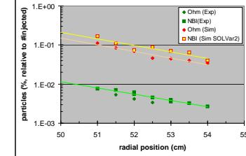
ERO modelled flux about 15 times larger than deposition observed on QMB
