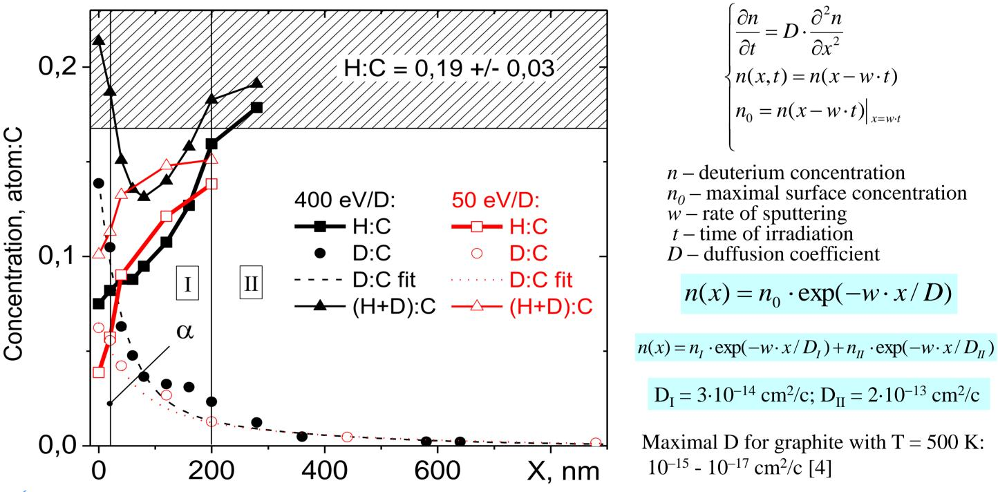
ions extracted from plasma. Irradiated C:H films were sputtered by argon ions in the range of 20 nm to 900 nm and then analysed by TDS method. A number of such experiments were carried out. As a result depth profiles of hydrogen isotope distribution in C:H films have been obtained.
