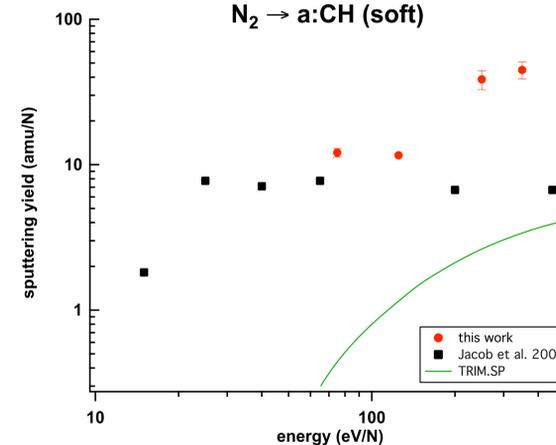
Comparison of the obtained steady-state sputtering yields for the impact of  $\text{N}_2^+$  ions on soft a-C:H with previous data [2] for hard a-C:H and the results of TRIM.SP calculations (physical sputtering only) for a carbon surface [6]. Both sputtering yields as well as energies are normalized to the number of incident N atoms.
