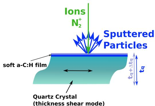
Schematic drawing illustrating the basic concept of a quartz crystal microbalance. Total mass changes of the target film are detected in situ via changes in the resonance frequency of a quartz crystal driven at its thickness shear mode.
