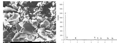
SEM micrograph and EDS spectrum of dust collected from divertor plate 2.
