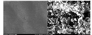
SEM micrographs of the initial divertor plate 1 and after campaign 2006-2009. The traces of graphite brittle fracture are marked by a circle.
