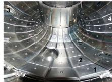
Lower part of Globus-M. RTi divertor tiles (0.85 m<sup>2</sup>) assembled inside vacuum vessel. Figures show the places of dust collected.
