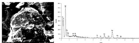
SEM micrograph and EDS spectrum of spongy particles with the size up to 100 microns. The spongy particles consisted of boron, carbon and oxygen with the characteristic form of "cauliflower". Formation of such particles was connected with flaking of deposited layers. The layers are formed during vacuum vessel conditioning and boronization in helium glow discharge.
