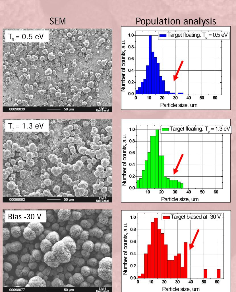
Formation of large (D>30 µm) dust particles at higher energies
