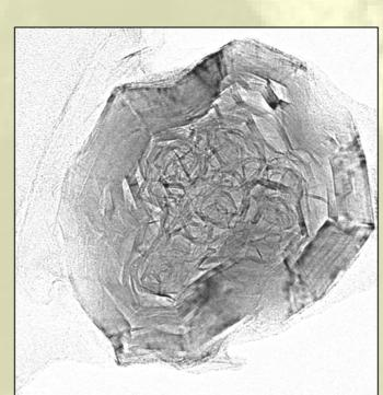
TEM images reveal presence of nano-sized conical structures as well as spherical nanoparticles on plasma exposed surfaces. Onion shape of the latter suggests formation in the plasma
