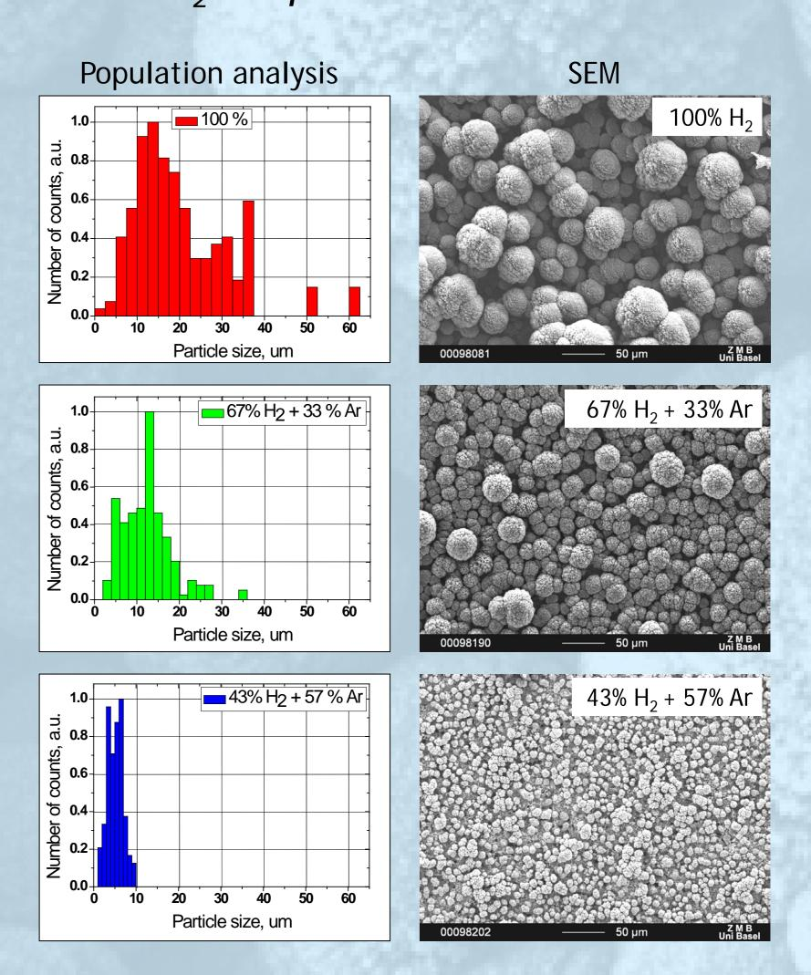
Addition of argon into the hydrogen plasma beam shifts the particle size distribution towards smaller values (D<sub>max</sub>≤10 µm)
