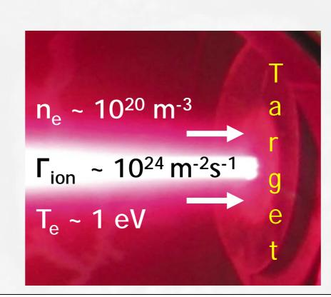
Operation in hydrogen, hydrogen/argon, nitrogen
