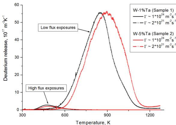
Low-flux exposures - from Y. Zayachuk, et al., Fusion Eng. Des. (2011), doi:10.1016/j.fusengdes.2011.03.094
