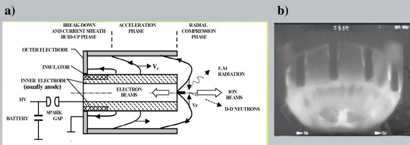
Figure 2) a) Evolution of the plasma inside of the gun and b) plasma picture at pinch.
