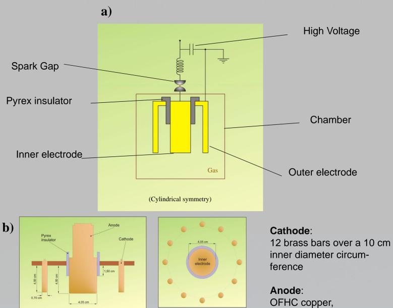
Figure 1) a) Schematic Diagram of the “gun” and electric wiring. b) The anode is made of a OFHC copper cylinder, while the cathode is made out of 12 OFHC copper bars. [1]
