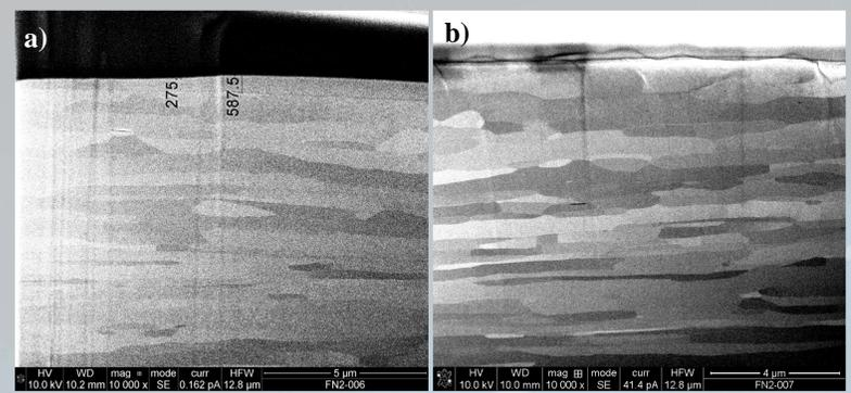
Figure 5) Cross-section images at 10000X of W-samples a) after 25 shots with deuterium b) 30 shots with He
