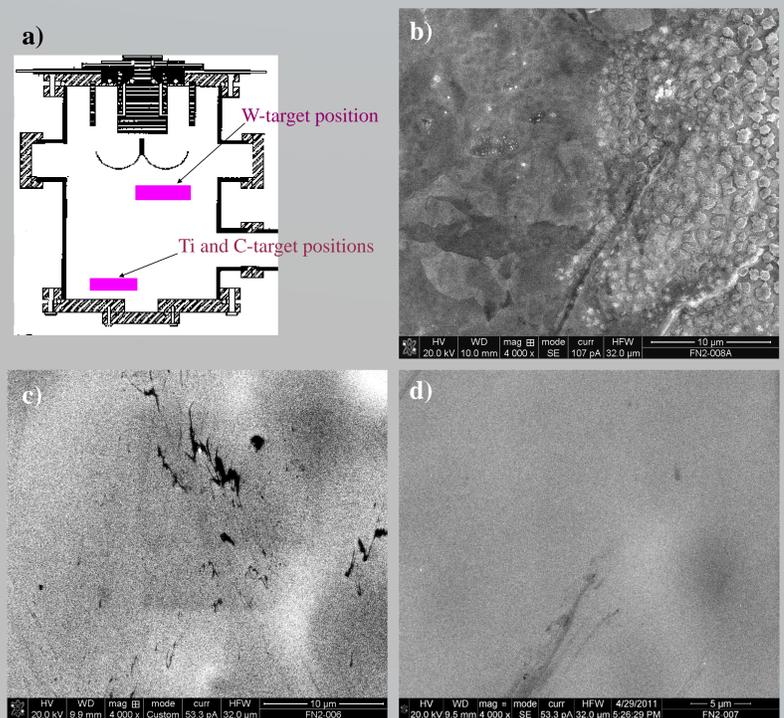
Figure 4) a) Schematic diagram of the position of the targets. b) image of sample as supplied c) Sample after 25 shots with deuterium d) sample after 30 shots with He.
