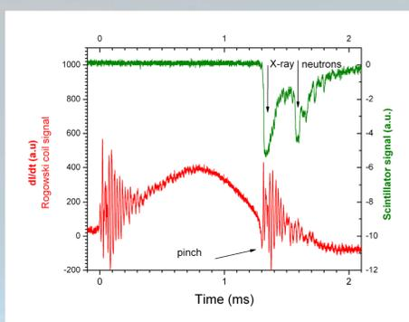
Figure 3) Typical Rogowski coil and scintillator signals for a deuterium discharge
