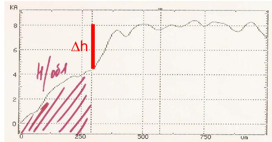
Radiation-induced linear deformation  $\Delta H$  (swelling) vs dose of the 5 MeV  $^{12}\text{C}^+$  carbon ion for pyrographite, MPG-8 and SEP NB-31 after cyclotron
