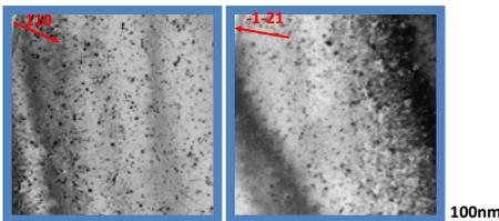
Effect of grain orientation: Loop coalescence is significantly favoured in (113) grain orientation.
