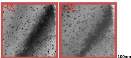
Effect of material purity: Loop size increases, density decreases with the increase of purity level.
