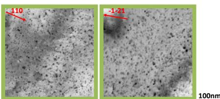
Effect of alloying element Re: Re suppresses loop growth and coalescence.
