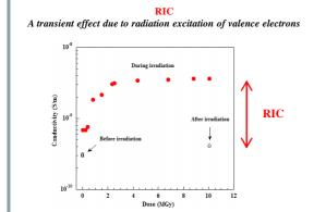
The initial conductivity rapidly increases at the on-set of irradiation from 3 to 7 x 10<sup>-10</sup> S/m, and then more slowly reaching 3.6 x 10<sup>-9</sup> S/m by 10 MGy. The measured RIC at 10 MGy (3.2 x 10<sup>-9</sup>) is small and suggests a high concentration of defects and/or impurities in the material, which act as carrier recombination sites.
