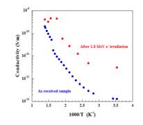
Electrical conductivity of the  $\rm Er_2O_3$  coating was measured from 10 to 450°C, before and after 4 hours (10 MGy) of 1.8 MeV electron irradiation at 450°C. An increase is observed in the electrical conductivity, more pronounced at low temperatures. This type of increase is typical for RIED.
