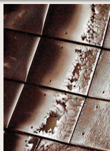
Flaking of co-deposited layer on lower part of limiter, TFTR, Nov 1998
