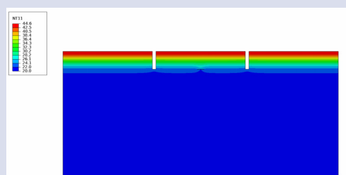
Figure 6 Transient Heat Transfer Analysis of Heat Pulse in Abaqus
