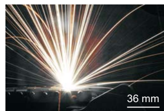
Fig. 8: Heavy brittle destruction, absorbed power density 316 MW/m 2 , 1 ms, first shot, room temperature
