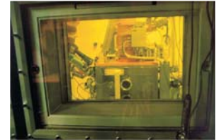
Fig. 2: Electron beam material test facility JUDITH 1 (Juelich Divertor Test Facility in Hot Cells)
