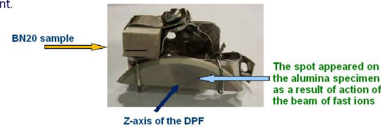
Fig. 10 A picture of the specimens' fixation BN on the top left and Al 2 O 3 on the bottom; see the semicircular dark spot on it - the result of irradiation by the axial beam of fast ions
