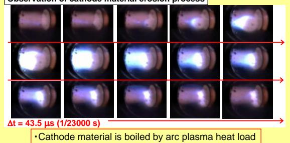
Cathode material is boiled by arc plasma heat load
