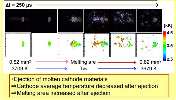
Ejection of molten cathode materials
