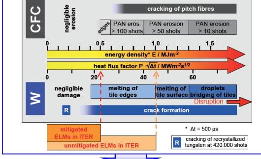
It is essential to study the interaction of high heat flux plasmas of ~GW/m<sup>2</sup> with refractory metal target
