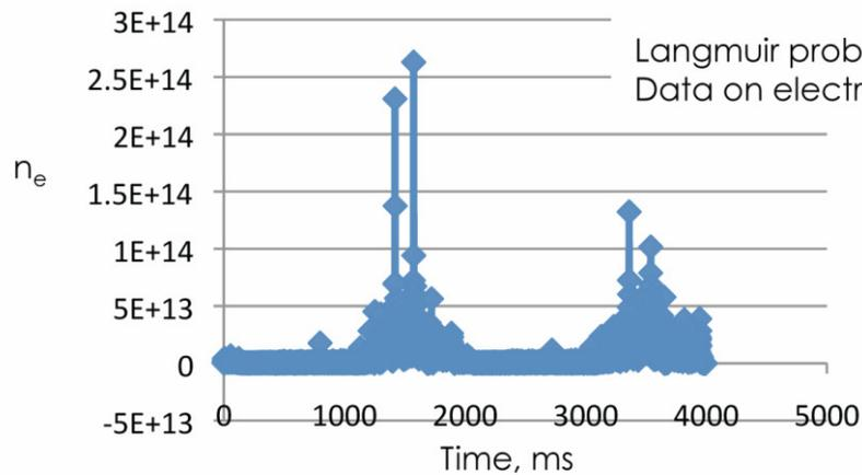
Added neutron beam injected at 2000 ms, plasma ended with disruption  $\sim 3100$  ms but migrated upward, no thermal dump on DiMES
