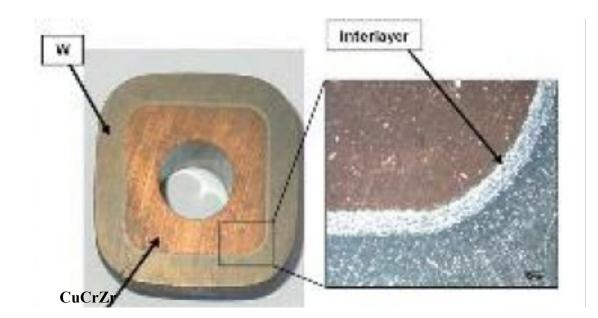
This coating/interlayer/ substrate combination has been successfully tested under thermal fatigue tests performed at the electron beam facility FE200 (Le Creusot-France). The mock up with 5 mm thick W coating realised with the low pressure plasma spray technique withstood heat fluxes up to 5 MWm<sup>-2</sup> in cooling conditions relevant for ITER.
