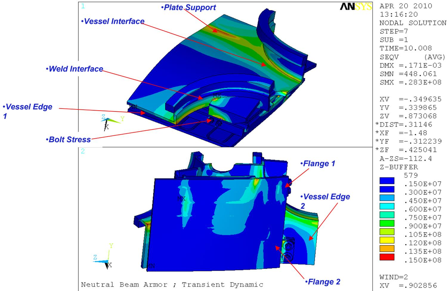
•The Transient Equivalent Stress at Max Current is less than 10 Ksi
