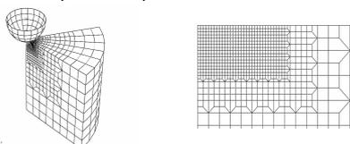
Fig. 2. FEM model: partial FEM domain (left) and details of the mesh at the region of contact (right).
