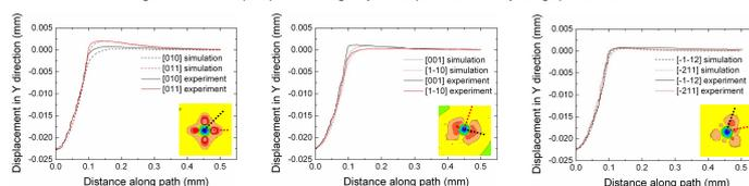
Fig. 15. Comparisons of the section profiles of imprints on all three orientations
