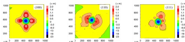
Fig. 13. Experimental imprint profiles of single crystal samples of different crystallographic orientations.
