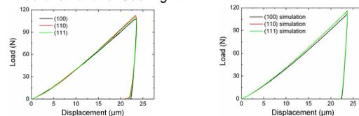
Fig. 11. Experimental and numerical load-displacement curves on single crystal samples of different crystallographic orientations.
