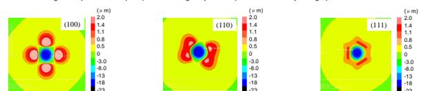
Fig. 14. Numerical imprint profiles of single crystal samples of different crystallographic orientations.
