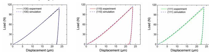
Fig. 12. Comparisons between experimental and numerical load-displacement curves on single crystal samples of different crystallographic orientations.
