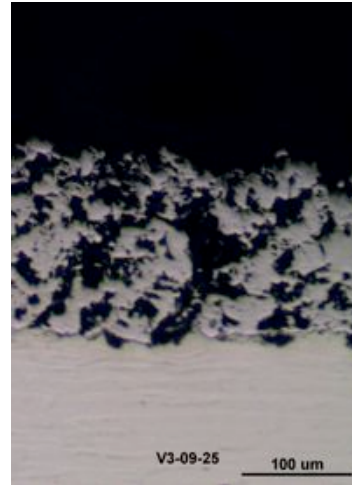
LLD surface cross section: plasma sprayed porous Mo on stainless with Cu backing plate
