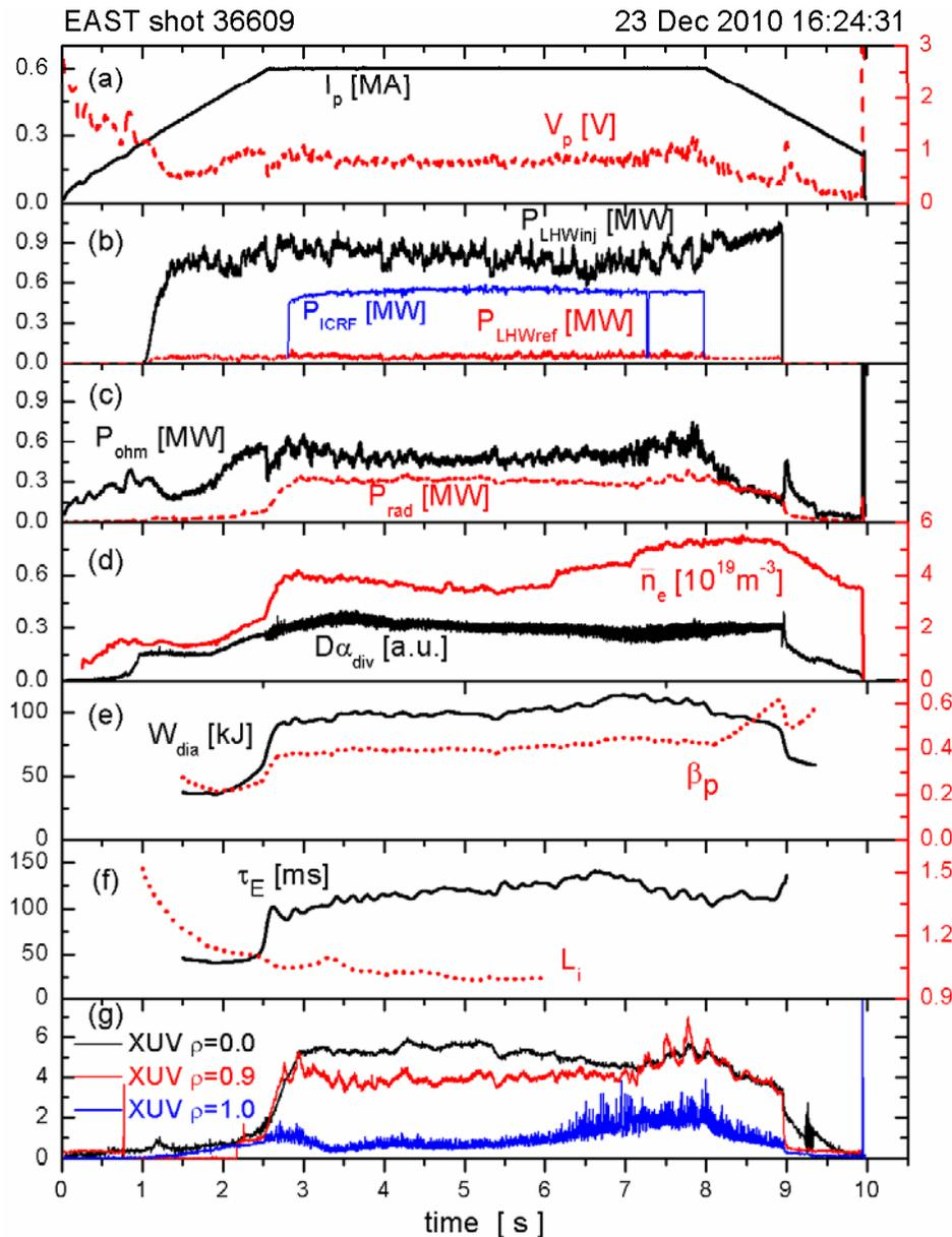
**Power:** LHCD 2.45GHz, 1.3MW, ~14% transmission line loss; ICRF 20-70MHz, 1MW, effective coupling < 0.5 MW
