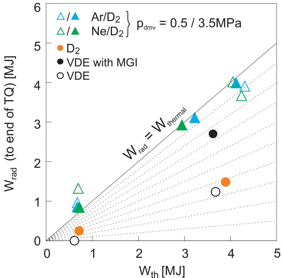
significant amount of  $W_{\text{thermal}}$  is radiated
