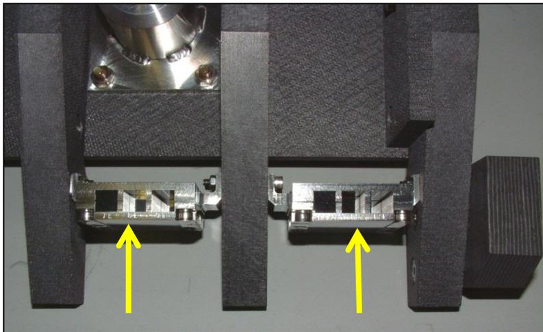
Mirrors installed on the outer divertor carrier
