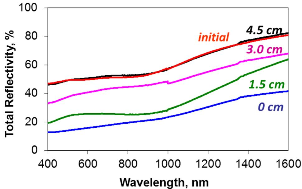
**Divertor:** Reflectivity loss for mirrors close to plasma is larger than deep in the channel.
