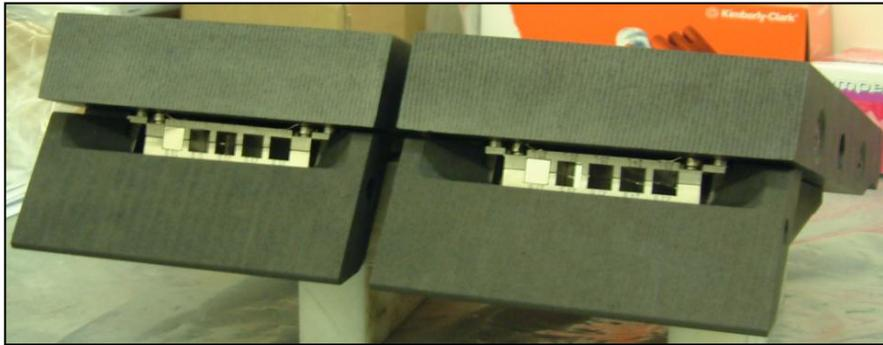
Mirrors in cassettes under the load bearing plate (divertor base)
