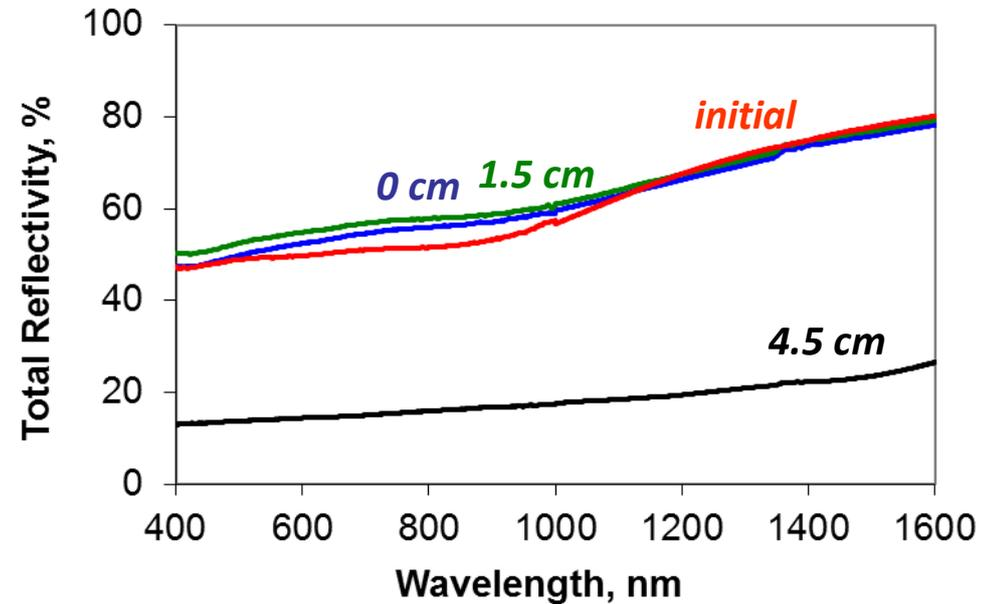
*No significant difference between mirrors protected and not protected by shutter.*
