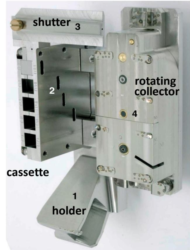
Bracket assembly for installation of mirrors and deposition monitors on the main chamber wall.
