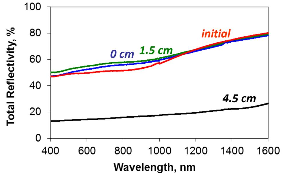
**Wall:** Reflectivity loss for mirrors close to plasma is smaller than deep in the channel.
