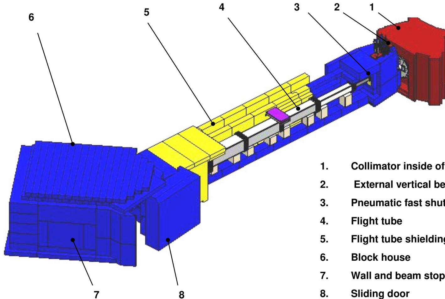
1. Collimator inside of the biological shielding
