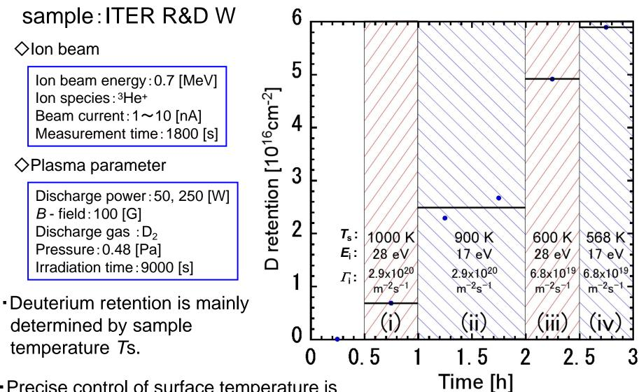
Precise control of surface temperature is required independently plasma condition.
