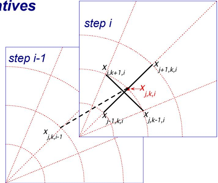
$f(\mathbf{x})$  generic function of position  $\xrightarrow{\text{at lowest order}}$   $\Delta f(\mathbf{x}) = \frac{\partial f}{\partial x_1} \Delta x_1 + \frac{\partial f}{\partial x_2} \Delta x_2 + \frac{\partial f}{\partial x_3} \Delta x_3$
