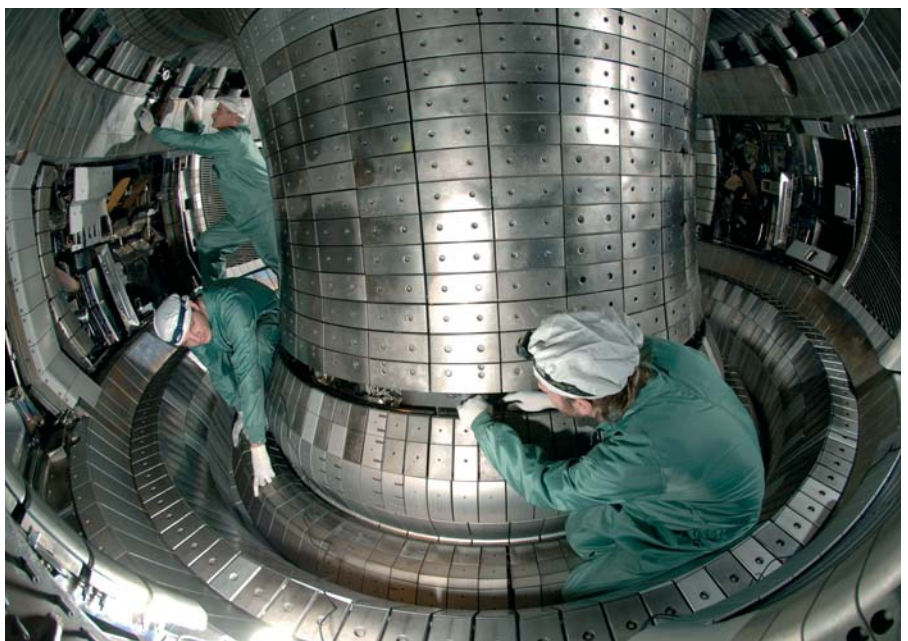
Fig. 2: Wide-angle view of the AUG inner wall with tungsten coated tiles.
