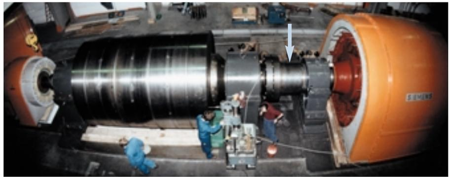
Fig. 5: Flywheel generator, position of torque sensors indicated by arrow.
