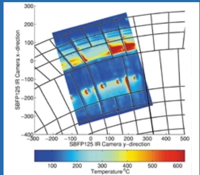
Fig. 3: Camera view of the target heat load pattern in the outer and inner upper divertor during a Type-I ELM.
