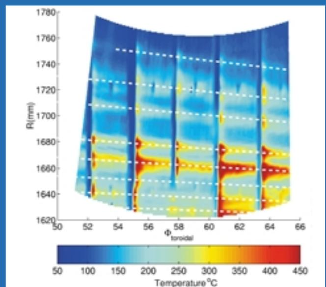
Fig. 4: Heat load pattern of the outer divertor target mapped onto target coordinates and overlaid with the intersection of 8 field lines starting at distinct toroidal positions in the outer midplane
