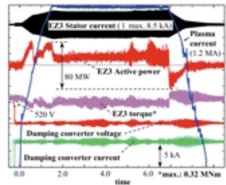
Fig. 6b: Active damping of SSR on generator EZ3 using a damping power of only 1 MW.
