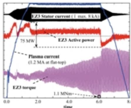
Fig. 6a: Measured generator current, active power and torque showing SSR on generator EZ3.
