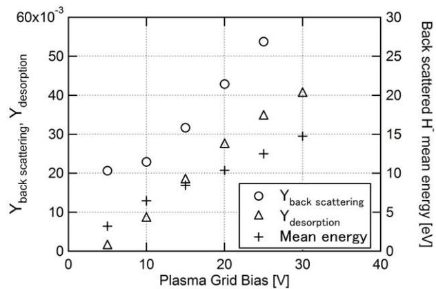
Figure 1. Probabilities to be reflected and desorbed as a  $H^-$  ion from cesiated metal surface. The plasma potential is assumed to be zero.
