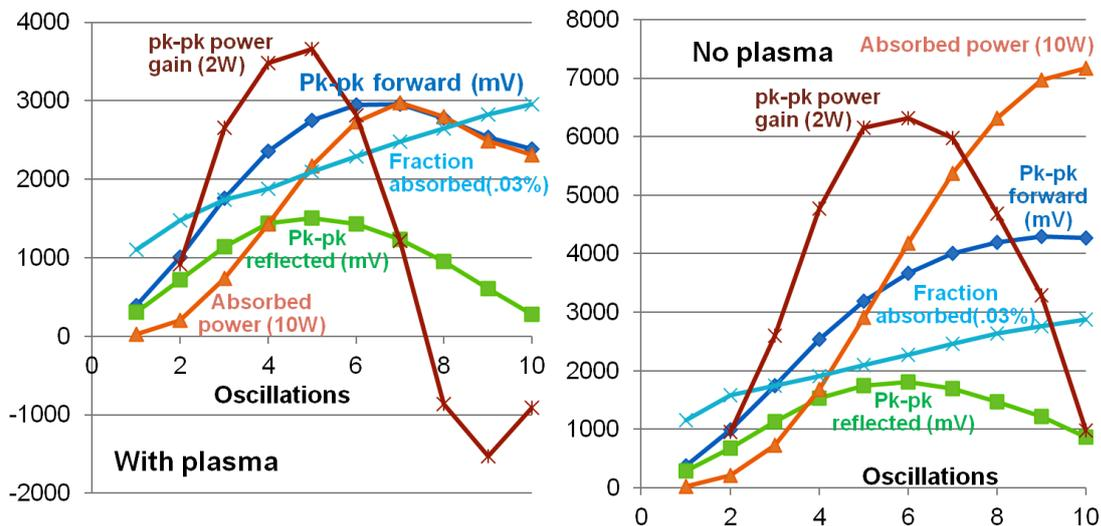
Figure 1. RF parameters of the first ten oscillations of the SNS  $H^-$  source with and without plasma.
