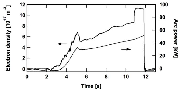
Figure 1. Time evolution of electron density measured with millimeter-wave interferometer.
