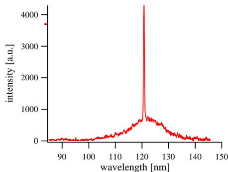
Fig. 1 The VUV spectrum of Lyman- $\alpha$  from a plasma excited by 14 GHz microwave
