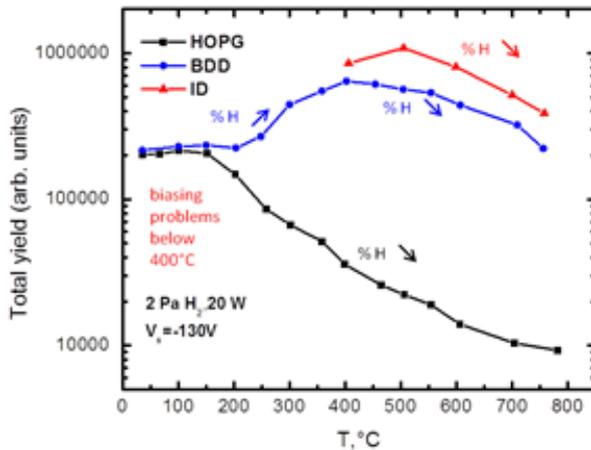
Figure 1. Temperature evolution of NI yields for different materials at 2.0 Pa H<sub>2</sub>, RF injected power of 20W and the surface bias of -130V.
