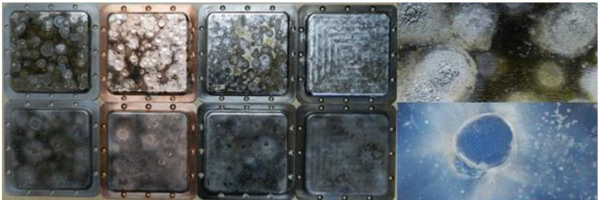
*Figure 1. Electrodes ( $10 \times 10 \text{ cm}^2$ ) after the tests. The top row are the anodes, the bottom row are the cathodes. From left to right: Stainless steel baked at  $800 \text{ }^\circ\text{C}$ , copper, titanium, molybdenum and a detail of the Ti electrodes. The detail on the right corresponds to a  $4 \times 2 \text{ cm}^2$  section of the Ti anode and cathode.*
