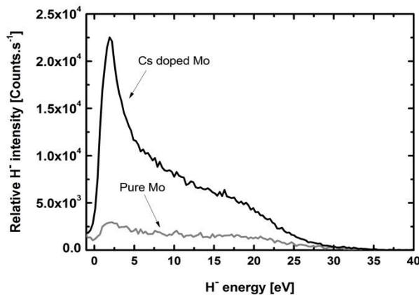
Figure 1. Comparison of the relative H<sup>-</sup> intensity of pure Mo (in grey) and Cs doped Mo (in black).
