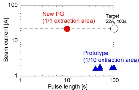
Figure 1. Progress of long pulse production by using temperature-controlled PG.
