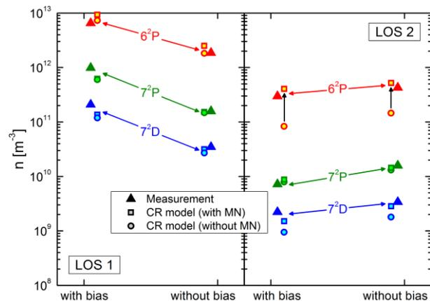
Figure 1. Measured and calculated population densities for three excited states in the Cs atom.
