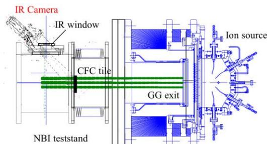
Figure 1. Schematic view of “MiniSTRIKE” installed at NIFS-NBI teststand.
