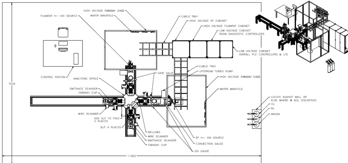
Figure 1. Plan view of the Ion Source Test Facility to be located at Buckley Systems factory in New Zealand.
