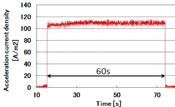
Figure 1. Acceleration current density for 60 s at 700 keV
