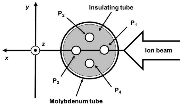
Figure 1. Cross-sectional view of the electrostatic probe.
