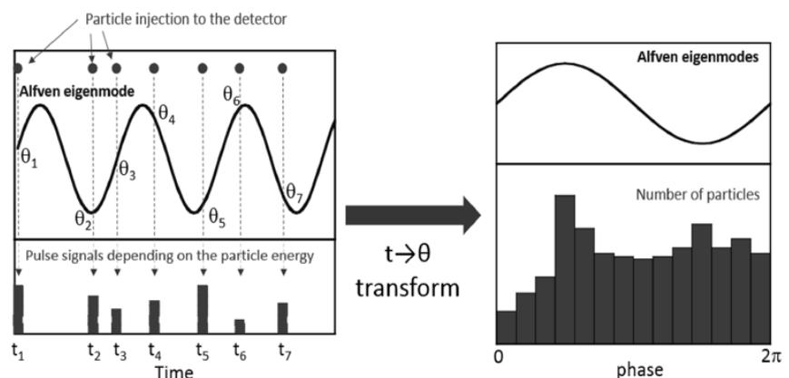
Fig. 1 Conceptual drawing of wave-particle interaction analyser (WPIA).
