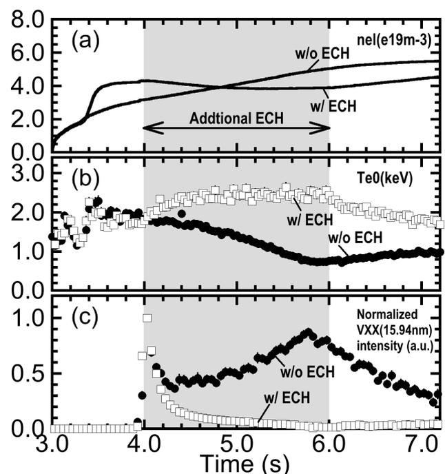
Fig. 1 Demonstration discharge of the mitigation of core impurity accumulation by applying the additional ECH (from  $t = 4.0$  s to  $t = 6.0$  s,  $P_{ECH} = 1.5$  MW,  $\rho_{abs} < 0.5$ ). As a guide, waveforms without applying the additional ECH are also shown. The tracer impurity, vanadium was injected at  $t = 3.95$  s by using the TESPEL technology.
