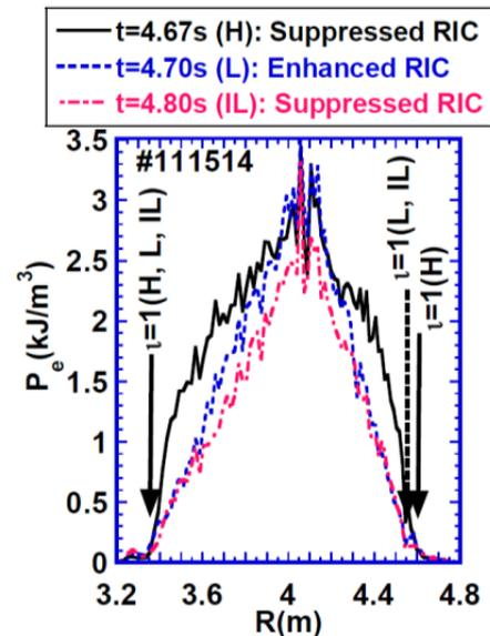
Fig.1 Comparison of electron pressure profiles in ELM-free H, L and IL phases of an H-mode in the specific magnetic configuration. The vertical arrows indicate the inferred  $\iota=1$  surface for three time slices.
