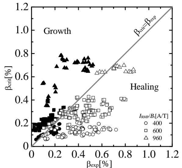
Fig. 1 Island healing transition boundary. Closed and open symbols indicate island growth and healing, respectively. Normalized RMP coil current  $I_{RMP}/B_t$  are 400A/T (circle), 600A/T (square), and 960A/T (triangle), respectively.
