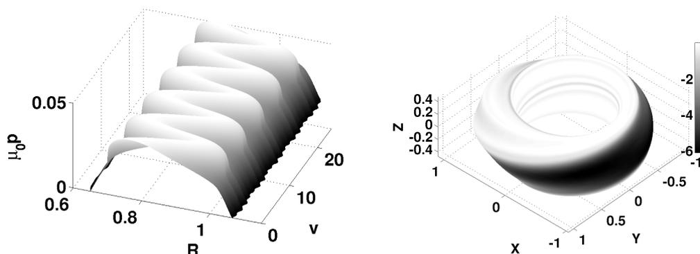
*Fig. 1. (Left) The pressure at the midplane over 5 toroidal transits constitutes a manifestation of a saturated ideal internal  $n = 1$  kink. (Right) The  $\sqrt{g}j_{\parallel}^2$  distribution on a surface close to the edge of the plasma corresponds to a saturated ideal external  $n = 1$  peeling/kink structure with the characteristics of an EHO or an Outer Mode (OM) [3].*
