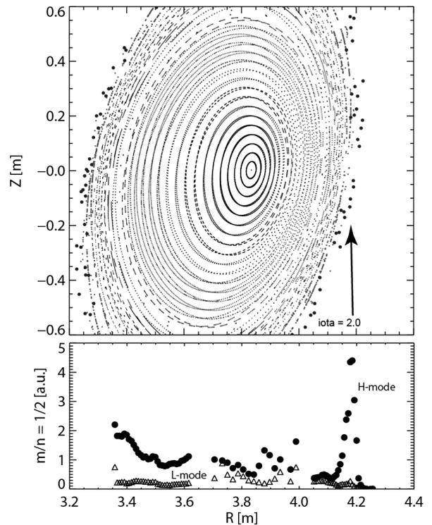
Fig. 1: Poincarre map of the magnetic field estimated by HINT2 and the fluctuation amplitude of the  $m/n = 1/2$  MHD instabilities measured by the CO<sub>2</sub> laser imaging interferometer.
