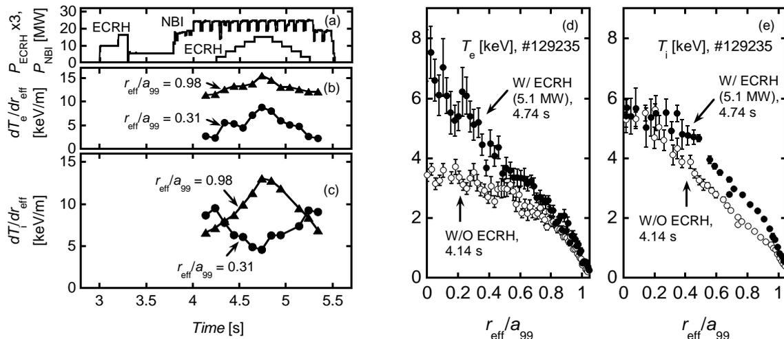
Fig. 1. The time evolution of (a) NBI and ECRH power, (b), (c) the gradient of  $T_e$  and  $T_i$  at  $r_{\text{eff}}/a_{99} = 0.31$  and 0.98, and the radial profiles of (d)  $T_e$  and (e)  $T_i$  before and during ECRH superposition.
