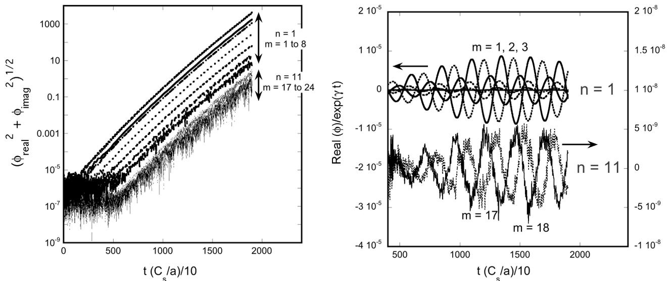
Figure 1 – (a) Amplitude growth, and (b) Alfvénic frequency oscillations  $\times exp(-\gamma t)$  vs. time, showing mode coupling between  $n = 1$  and  $n = 11$  components, as expected for an  $N_{fp} = 10$  field period stellarator.
