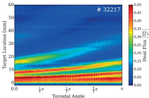
2D divertor heat flux profile for ASDEX Upgrade #32217 with rotated MP ( $n=2, 1$  Hz), measured with a new infrared system.
