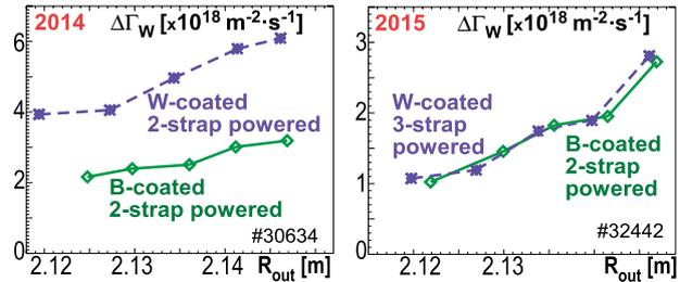
ICRF-specific W source at the W-coated antenna side limiter versus the outer plasma position, with the B-coated antennas as reference.
