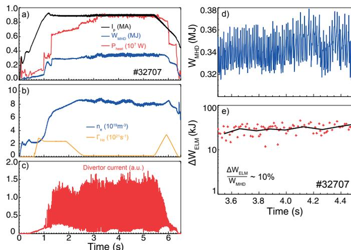
Time traces of an ITER baseline scenario in helium: (a) plasma current, stored energy and heating power, (b) line-averaged density and fuelling rate, (c) divertor current as ELM signature. Zoom of stored energy (d) and ELM energy loss (e).
