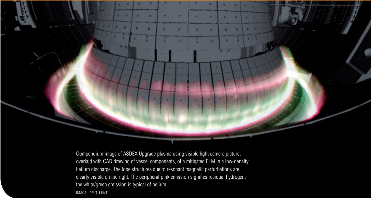
Compendium image of ASDEX Upgrade plasma using visible light camera picture, overlaid with CAD drawing of vessel components, of a mitigated ELM in a low-density helium discharge. The lobe structures due to resonant magnetic perturbations are clearly visible on the right. The peripheral pink emission signifies residual hydrogen; the white/green emission is typical of helium.
