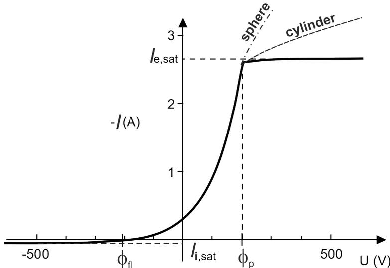
FIG. 1: Current-voltage characteristics of a Langmuir probe for different shapes of the probe head (from Ref. [23]).
