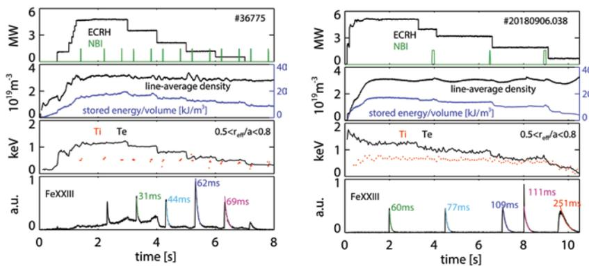
Representative time traces of comparison experiments at ASDEX Upgrade (left) and Wendelstein 7-X (right). From top to bottom, the applied heating power, the electron density and stored energy per volume, the average electron and ion temperatures for normalized radii between 0.5 and 0.8 and the observed levels of FeXXIII radiation are shown.
