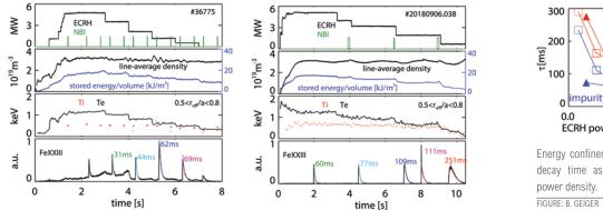
Representative time traces of comparison experiments at ASDEX Upgrade (left) and Wendelstein 7-X (right). From top to bottom, the applied heating power, the electron density and stored energy per volume, the average electron and ion temperatures for normalized radii between 0.5 and 0.8 and the observed levels of FeXXIII radiation are shown. FIGURE: B. GEIGER
