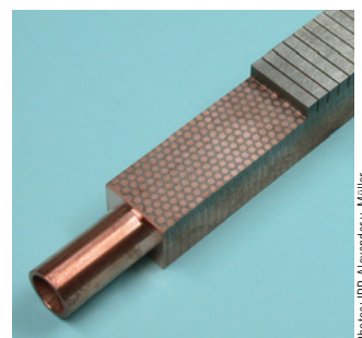
Mock-up of a plasma-facing component with a heat sink based on a copper-infiltrated tungsten honeycomb structure
