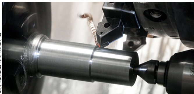
View into the lathe: Inconel 718 is dry machined with ceramic plates. The red-hot chips are removed – the bolts emerge.
