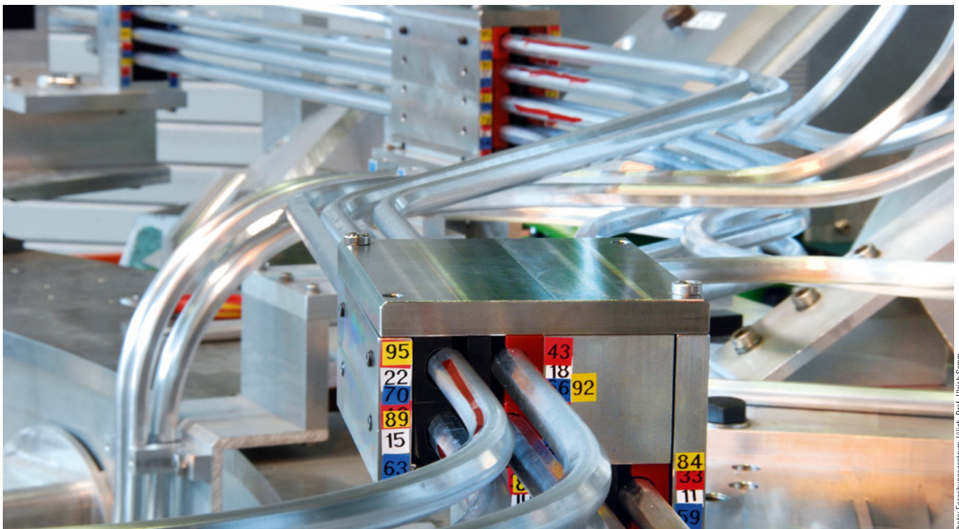
Geometric check of shaped superconductors
