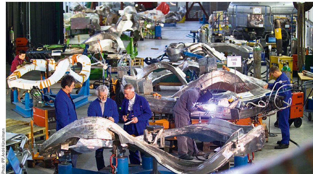
◀ Manufacturing of non-planar coils for Wendelstein 7-X ▼ Non-planar coil – here during “coil threading”
