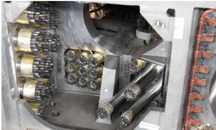
Wendelstein 7-X: Bolt connections on the central ring
