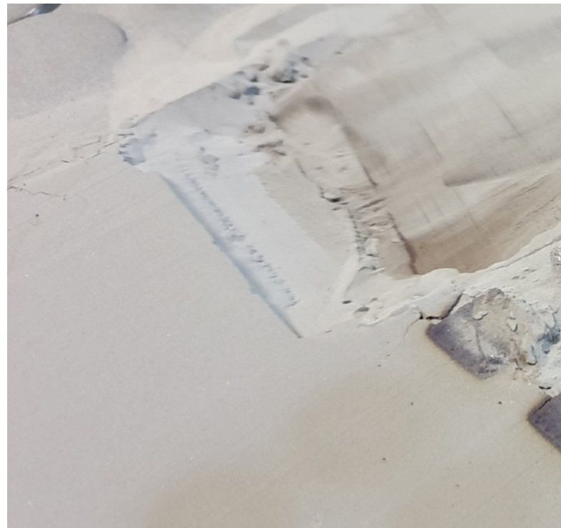
Additively manufactured tungsten parts after the manufacturing process when being removed from the powder bed.
