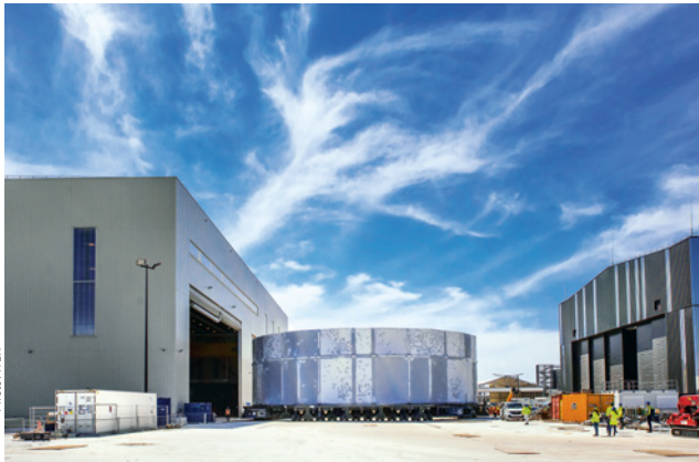
With the assembly of the ITER cryostat - here the “Upper Cylinder” – the Degendorf company once again demonstrates its know-how in complex stainless steel processing.
