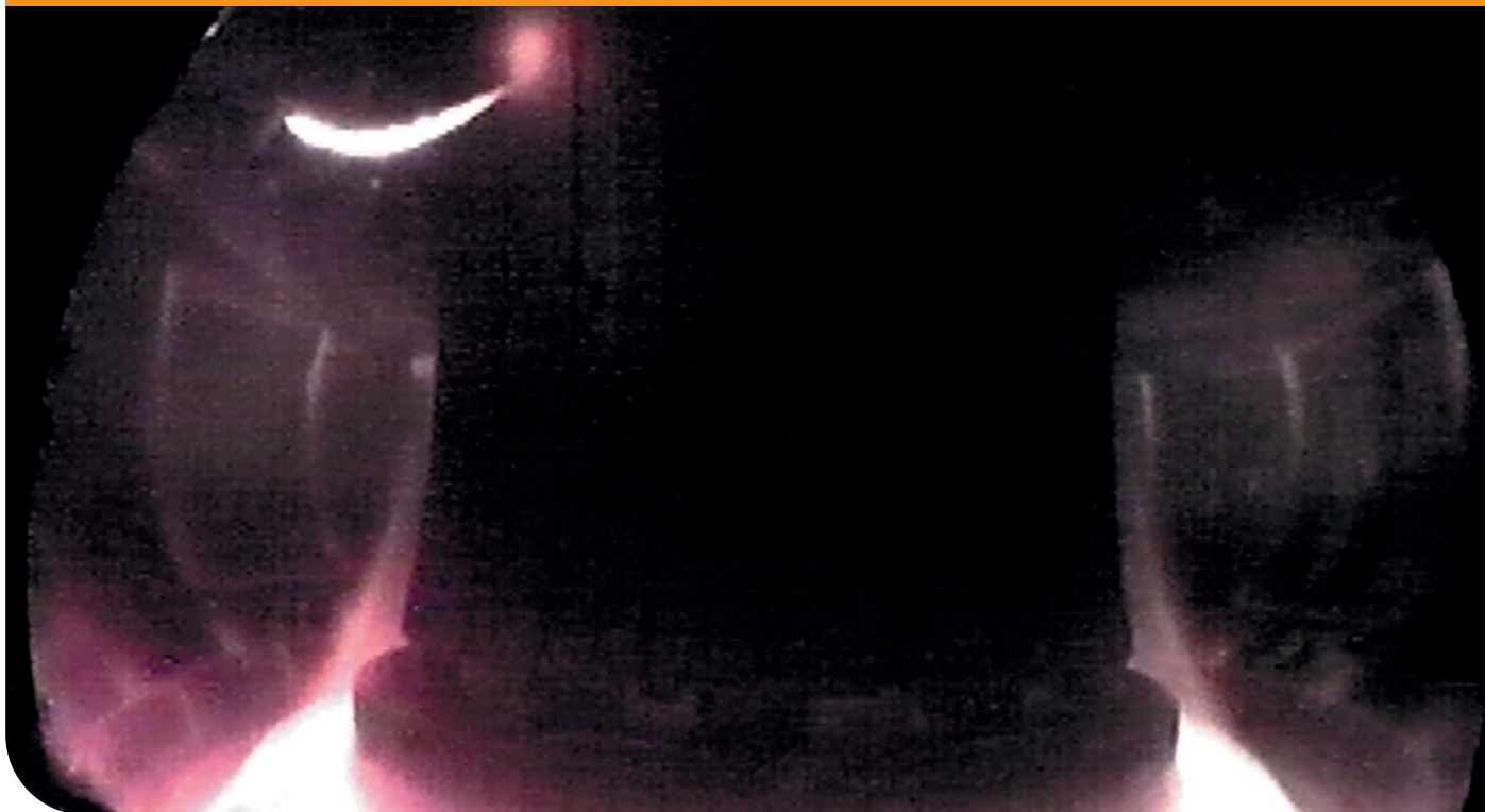
Fire and ice: an ultra-cold pellet produced from solid deuterium arrives in a hot ASDEX Upgrade plasma. While evaporating like a comet it serves for efficient particle fuelling.
