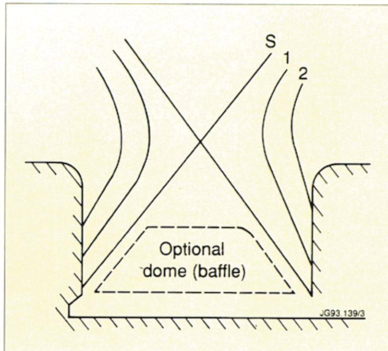
*Fig.53: Vertical target divertor with optional baffle*
