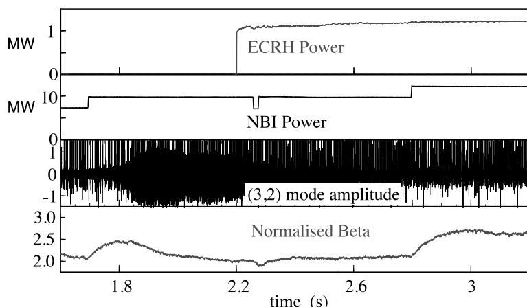
Fig. 8. Stabilization of neoclassical tearing modes with electron cyclotron current drive as indicated by the amplitude of the  $m = 3, n = 2$  magnetic perturbations. Value  $\beta_N = 2.6$  was achieved in steady state without these modes by raising the neutral beam power.
