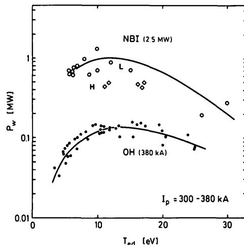
FIG.12. Total power loss onto divertor plates  $P_w = \int \gamma i_s T_{ed} d\vec{f}$  as calculated from ion saturation current  $i_s$  and electron temperature  $T_{ed}$  for discharges with Ohmic heating (OH) and 2.5-MW neutral-beam injection (NBI, L-type and H-type), respectively. Heat transmission rate is assumed to be  $\gamma = 7$ .
