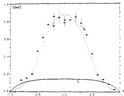
Fig. 13 Comparison of the calculated  $T_e$ -profile with the experimental data points. The calculated ion temperature is also given.
