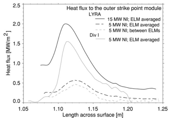
Fig. 10. Heat flux onto the outer divertor strike point module in the lyre-shaped divertor compared to DIV I.
