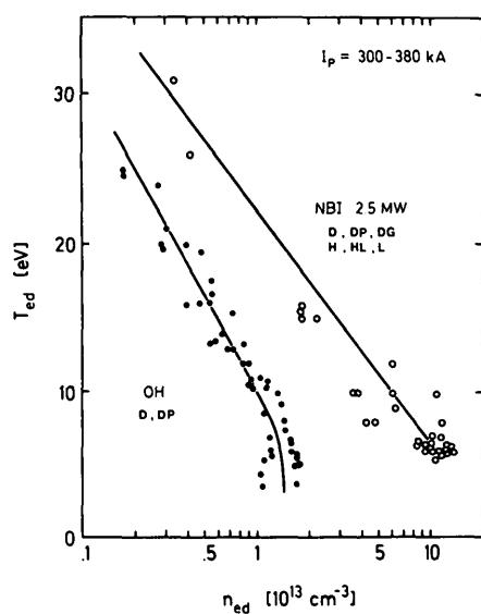
FIG. 10. Electron temperature in divertor  $T_{\text{ed}}$  versus density  $n_{\text{ed}}$  at constant heating power (OH: 0.3–0.4 MW, NBI: 2.5 MW) for various discharge modes: pumping (DP), no pumping (D) or gas puffing (DG) in divertor; L- and H-type discharges.
