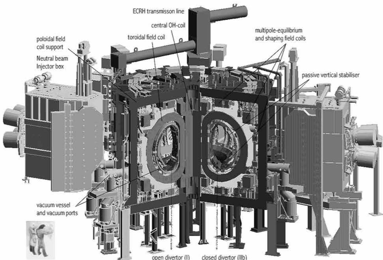
Fig. 1. Three-dimensional cutaway view of ASDEX Upgrade with heating systems and two different divertor configurations. Left: the open divertor I; right: the closed divertor IIb configuration.
