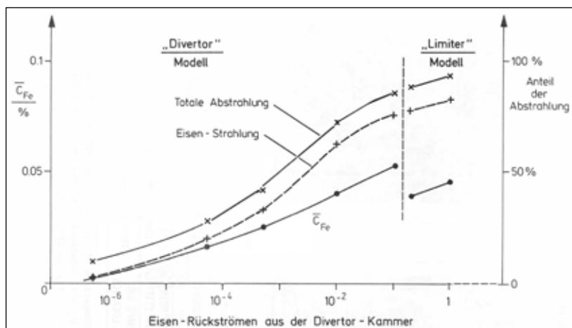
*Fig. 3 Dependence of Iron-concentration and radiative power losses on the impurity backflow fraction from the divertor chamber or the limiter, for a device with JET dimensions and power fluxes.*
