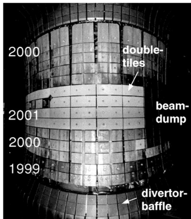
Fig. 4. The central column of ASDEX Upgrade with tungsten-coated tiles.
