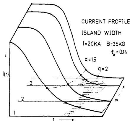
Fig. 3. Expected width of magnetic islands (hatched region) for various profiles of the OH-current distribution as they may result from the power deposition profile of NBI.
