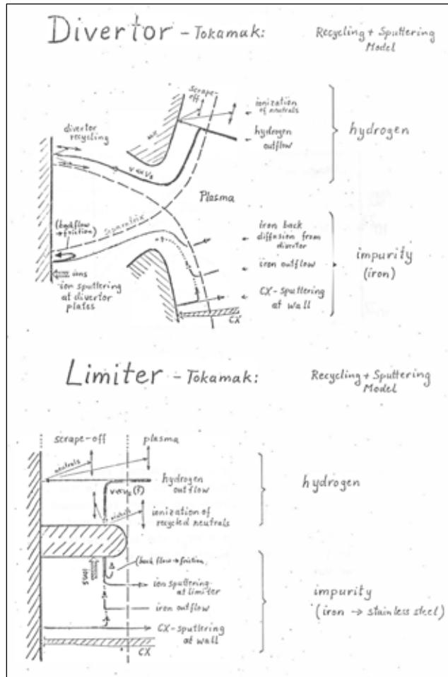
Fig. 2 Schematic representation of the processes contributing to the hydrogen and impurity household (here: iron) in a divertor and limiter tokamak.
