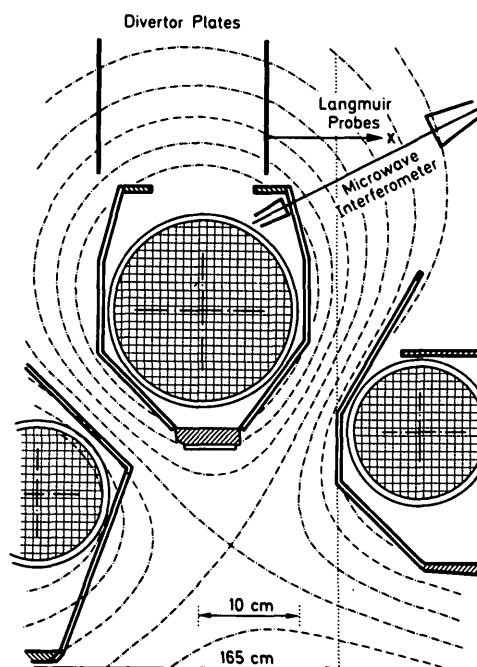
FIG. 1. Schematic drawing of divertor region indicating location of Langmuir probes and microwave horns.
