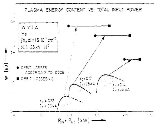
Fig. 4 Increase in plasma energy by NBI heating of OH target plasmas (hatched region). In all cases the curves indicate that the confinement time increases with the application of NBI.
