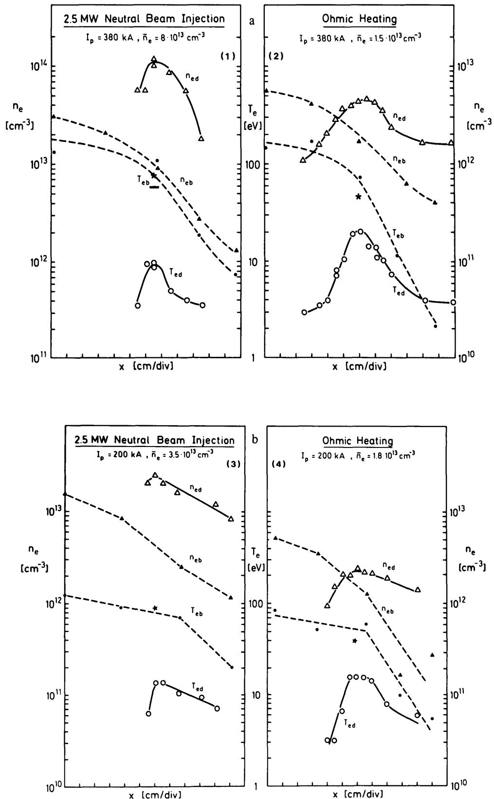
FIG.5. Radial profiles of electron density and temperature at torus mid-plane ( $n_{eb}$ ,  $T_{eb}$ ) and near divertor plate ( $n_{ed}$ ,  $T_{ed}$ ) for the four cases of Fig.4: (a) cases 1 and 2; (b) cases 3 and 4.
