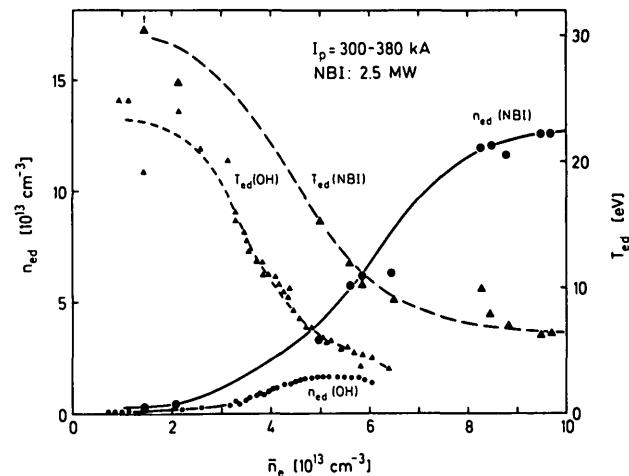
**FIG. 3.** Peak values of electron density  $n_{ed}$  and temperature  $T_{ed}$  near divertor plate as functions of bulk plasma density  $\bar{n}_e$  for discharges with Ohmic heating (OH) and 2.5-MW neutral-beam injection (NBI), respectively.
