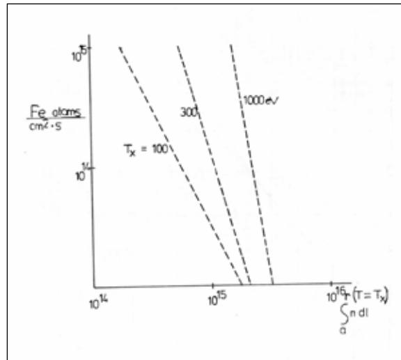
Fig. 8 Iron sputtering by CX neutrals as a function of the density line integral between wall and different isotherms. The lines shown are a composite result of various JET and ZEPHYR simulation runs. A sputtering rate of  $3 \times 10^{14}$  Fe-atoms/cm<sup>2</sup> · s corresponds to a yearly wall ablation of 1 mm.
