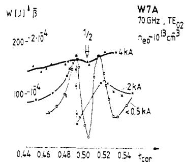
Fig. 15 Achieved plasma energy vs.  $t$  (a) for constant gyrotron power aiming at low beta. Shear is varied by small plasma currents. The values indicated are adjusted by proper selection of small loop voltages.
