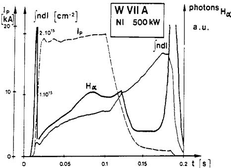
Fig. 6 Transition to net-current free, NBI-maintained operation. The decreasing  $H_\alpha$ -signal, inspite of the strongly increasing density, indicates an increase of the particle confinement by about a factor of five at  $t = 0.17$  s.
