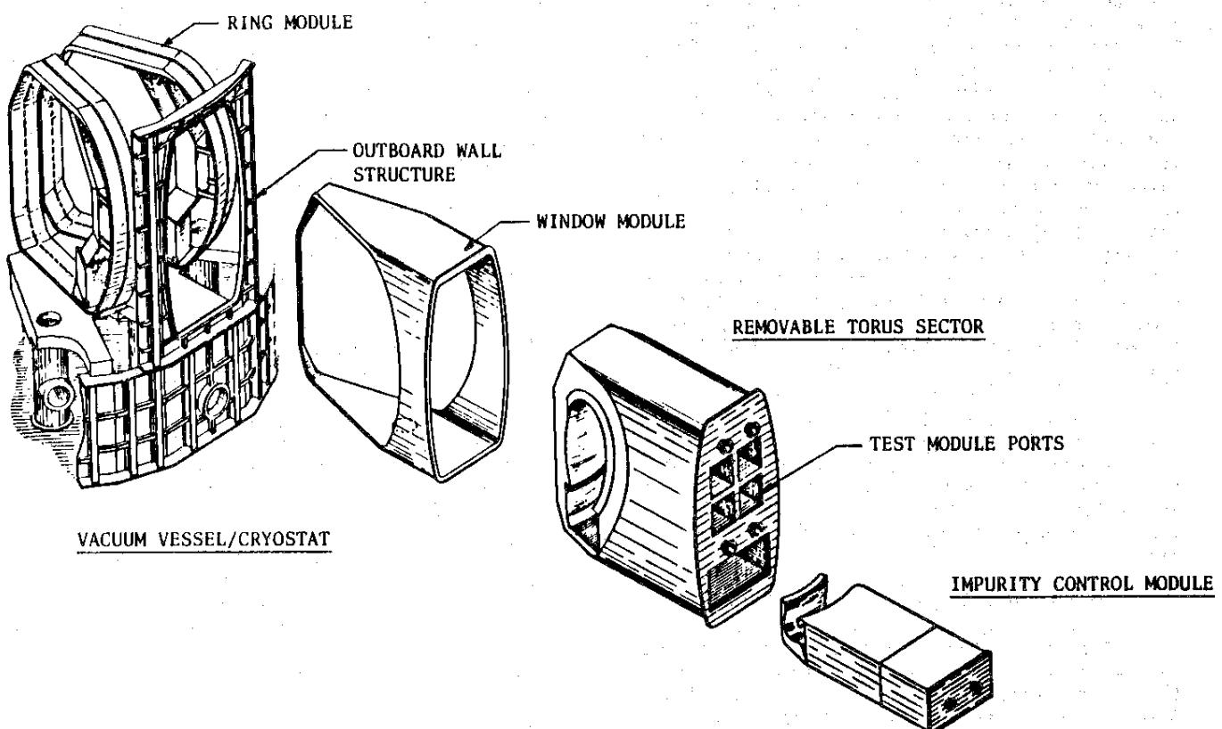
Fig. 4 INTOR maintenance concept.
