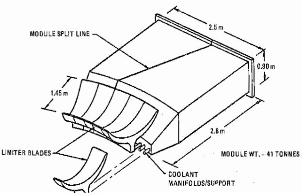
Fig. 3 Shaped, double-edged bottom limiter.
