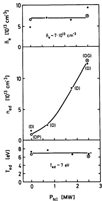
FIG.7. Control of electron temperature near divertor plate  $T_{ed}$  at low value ( $T_{ed} \approx 7 \text{ eV}$ ) even for high neutral-injection powers ( $P_{NI} \leq 2.5 \text{ MW}$ ) by changing recycling conditions in divertor (for fixed bulk plasma density,  $\bar{n}_e \approx 7 \times 10^{13} \text{ cm}^{-3}$ ).  $I_p = 380 \text{ kA}$ .
