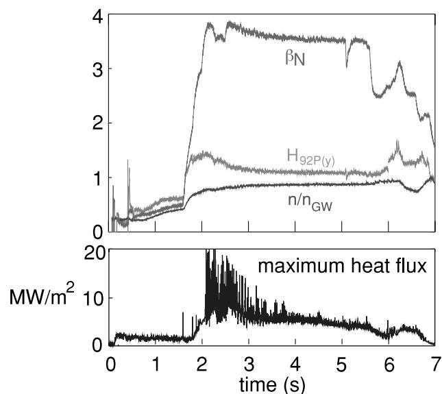
Fig. 7. High  $\beta_N$  discharge with reduced ELM activity as seen in a reduction of the maximum heat flux.
