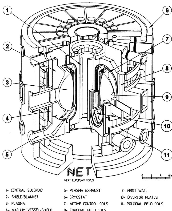
FIG. 1. Three-dimensional view of the NET device.
