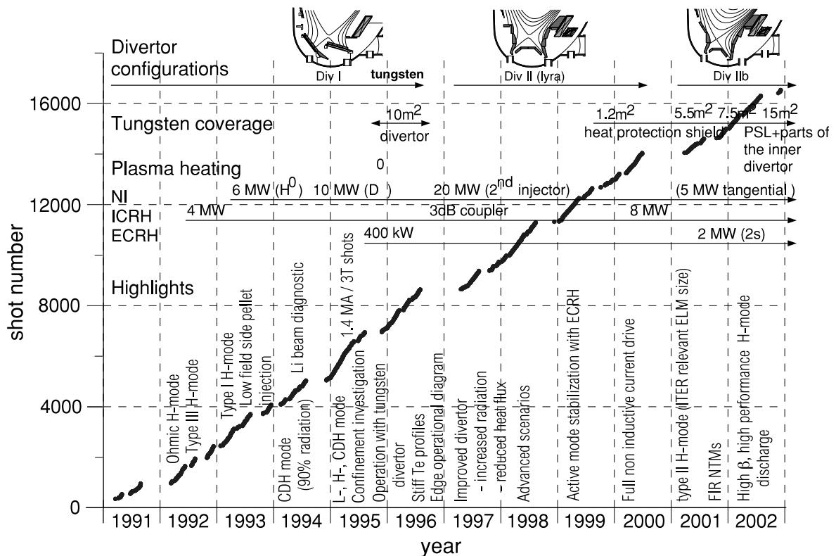
Fig. 3. Overview of ASDEX Upgrade operation. The gaps in the line for the accumulated number of shots mark shutdown periods. Major hardware changes, such as increased heating power and divertor modifications, are indicated. The main physical results and the start of program topics are mentioned in the lower part of the figure.
