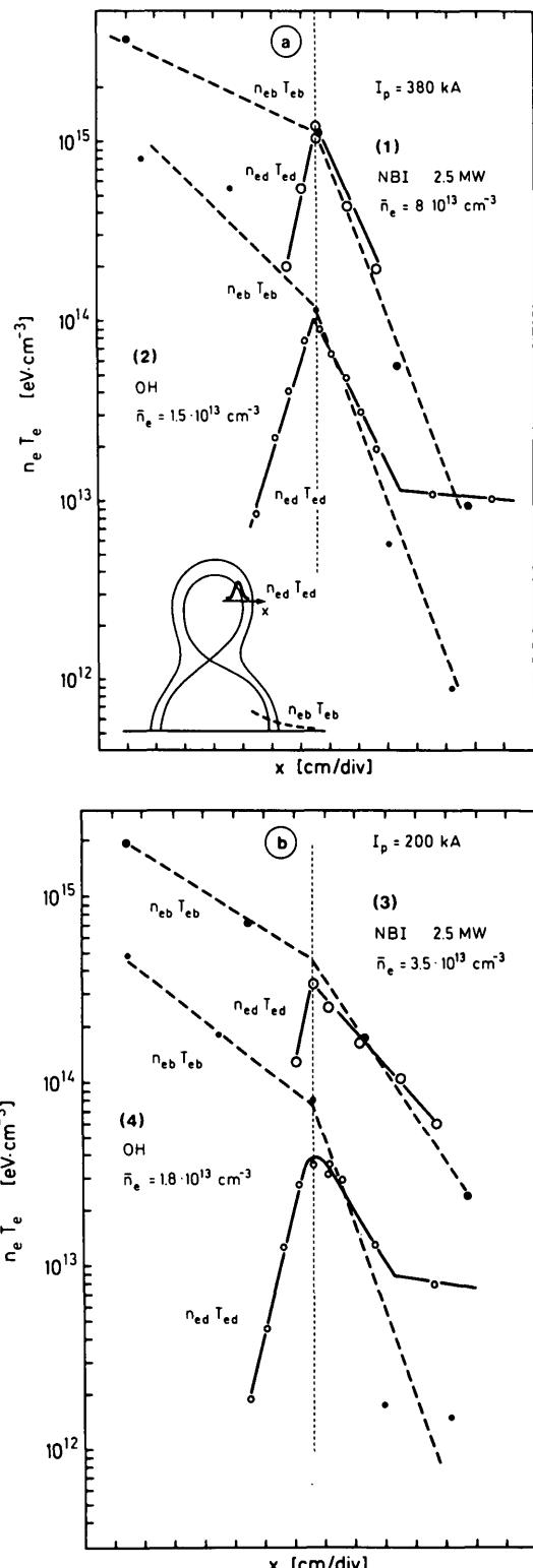
**FIG.4.** Radial profiles of electron pressure at torus mid-plane ( $n_e T_e$ ) and near divertor plate ( $n_{ed} T_{ed}$ ) for four typical cases: (a, 1) high-current, high-density discharge with  $P_{NI} = 2.5 \text{ MW}$ ; (a, 2) high-current discharge with  $P_{NI} = 0$ ; (b, 3) low-current discharge with  $P_{NI} = 2.5 \text{ MW}$ ; (b, 4) low-current discharge with  $P_{NI} = 0$ . Abscissa gives horizontal distance in the divertor. For torus mid-plane, distance is around 0.5 cm/div.
