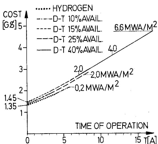
Fig. 8. Accumulation of INTOR operating cost. For three different machines designed for  $0.2$ ,  $2$ , and  $6.6 \text{ MWa/m}^2$  and staged operation as indicated in the insert. The intersection with the ordinate at  $T = 0$  gives the direct capital cost of these devices.
