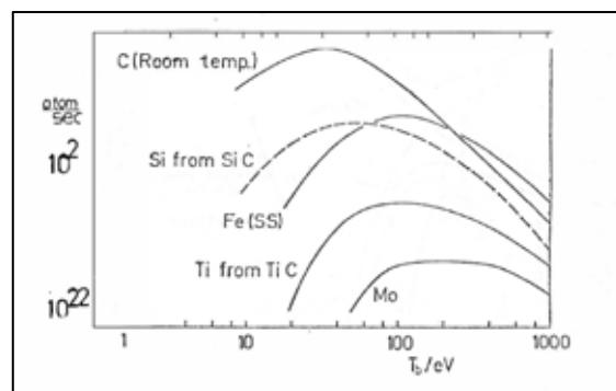
*Fig. 1 Sputtering rate for a 3 GW thermal reactor in case of energy transfer to the walls via particle motion. Every ion impact is assumed to be accompanied by a total energy transfer (electron + ion) of 4 kT<sub>b</sub>; the acceleration in the potential sheath is not taken into account.*
