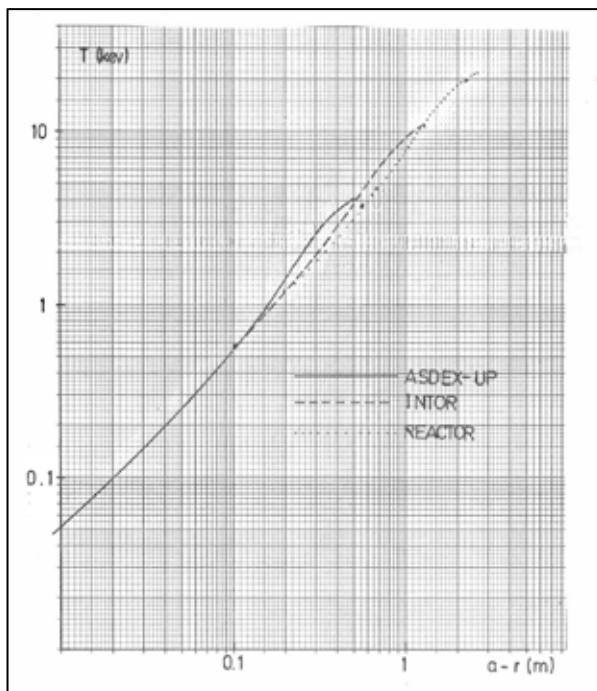
*Fig. 7 Temperature profiles for identical heat flux through the boundary, for experiments of different size (obtained under the assumption of peaked, similar heat deposition profiles and a heat conduction law of the form  $n\chi = f(T)$ ).*
