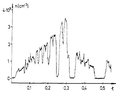
Fig. 1. Confinement vs. twist number  $t$  for a barium plasma in the shearless Stellarator W III-A. For constant input flux of barium plasma the resulting density is a direct measure of the confinement time.
