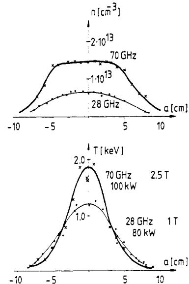
Fig. 10 ECF produced net-current free discharges for two cases: 28 GHz at 1 T and 70 GHz at 2.5 T. One immediately observes the difference in gradients. Please note that the particle source is at the edge but the power source at the plasma center.
