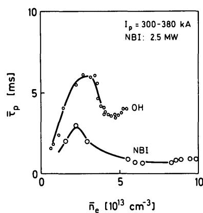
FIG.11. Global particle confinement time  $\bar{\tau}_p$  as function of bulk plasma density  $\bar{n}_e$  for Ohmically (OH) and neutral-beam-(NBI)-heated discharges.
