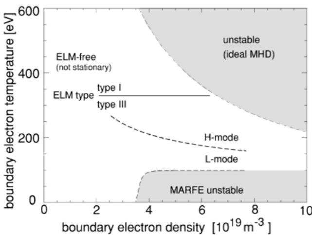
Fig. 9. Edge operational diagram for low triangularity configuration showing regime boundaries. Values  $T_e$  and  $n_e$  are taken 2 cm inside the separatrix to represent absolute values as well as gradients.
