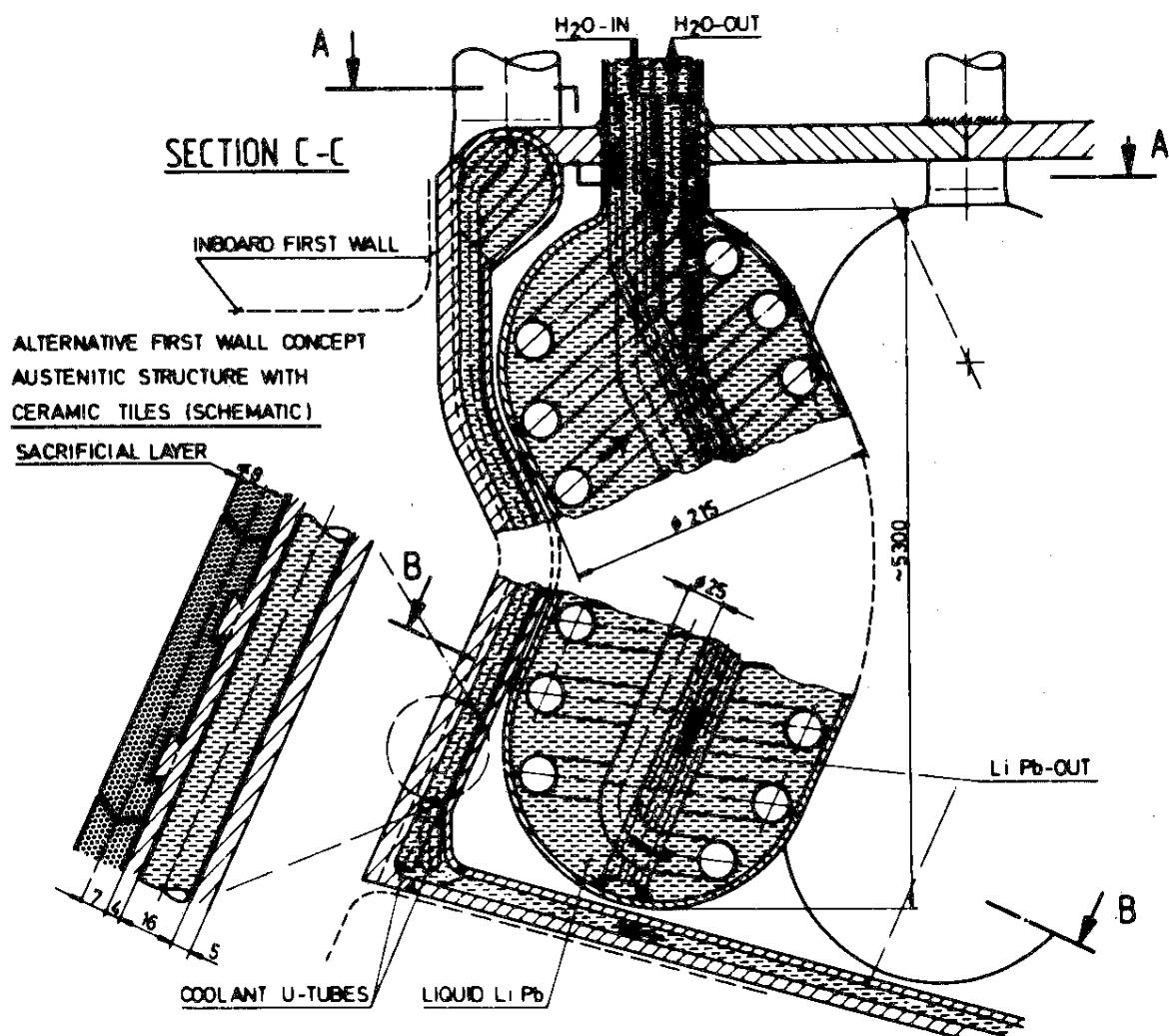
Fig. 6. Alternative first wall and blanket concept.
