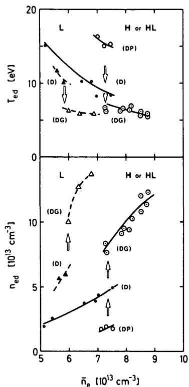
FIG.6. Variation of electron temperature  $T_{ed}$  and density  $n_{ed}$  near divertor plate for various recycling conditions in divertor: pumping (DP), no pumping (D) or gas puffing (DG) in divertor chamber. L and H denote L- and H-type discharges. Discharges at  $I_p = 300 - 380 \text{ kA}$  with 2.5-MW neutral-beam injection.
