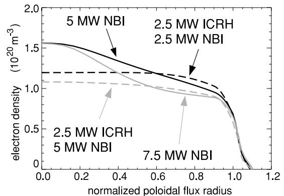
Fig. 6. Central heating (in this experiment by ICRH) results in flat profiles. The profiles taken from deconvolution of interferometry and lithium beam.
