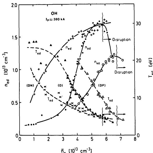
**FIG. 8.** Electron temperature  $T_{ed}$  and density  $n_{ed}$  near divertor plate as functions of bulk plasma density  $\bar{n}_e$  for various recycling conditions in divertor chamber: pumping (DP), no pumping (D) and narrowing divertor slit width from 6.5 to 3.7 cm (DN). Ohmically heated discharges with  $I_p \approx 380$  kA. For DN discharges, filling gas is hydrogen.
