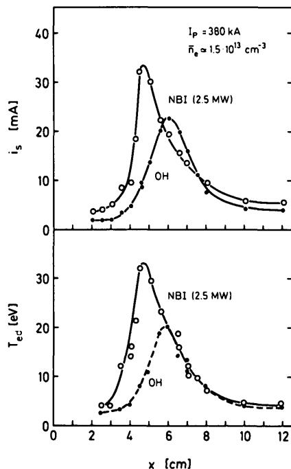
**FIG. 2.** Typical profiles of ion saturation current  $i_s$  and electron temperature  $T_{ed}$  in divertor for rather low-density discharges ( $\bar{n}_e \approx 1.5 \times 10^{13} \text{ cm}^{-3}$ ) with Ohmic heating (OH) and 2.5-MW neutral-beam injection (NBI), respectively. Distance  $x$  is counted from collector plate.
