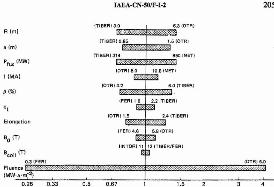
FIG. 1. Relative span of the parameters covered by the designs.
