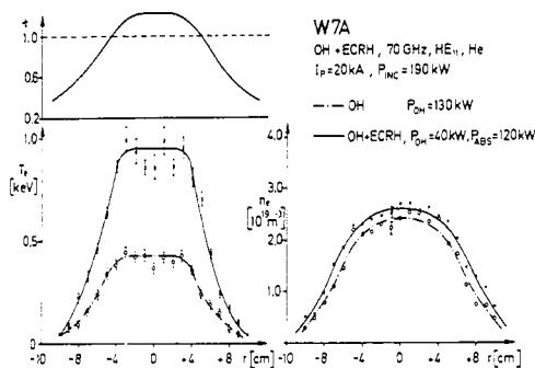
Fig. 5. Comparison of an OH-plasma without and with additional ECRH. The increase in plasma energy indicates a substantial increase of the confinement time for ECRH.
