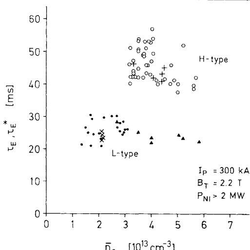
FIG. 2. Global energy confinement time vs average line density for toroidal limiter (triangles) and divertor discharges (other symbols).  $\tau_E$  (plusses and crosses) is deduced from thermal profiles and  $\tau_E^+$  (open circles, solid circles, and triangles) is determined from the diamagnetically measured  $\beta_{p\perp}$ .
