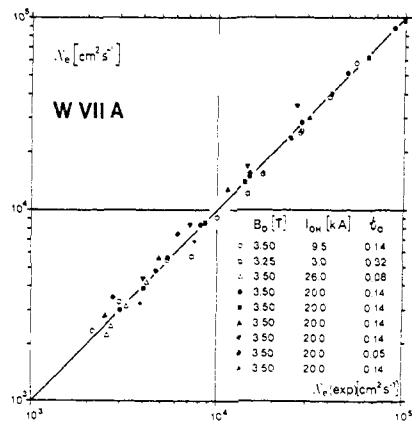
Fig. 2 Electron heat conduction for OH-plasmas in W VII-A for regions free of tearing modes and sawteeth.
