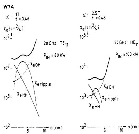
Fig. 11: Electron heat transport coefficients for the two discharges shown in Fig. 10. The bold trace is the sum of the three contributions:
