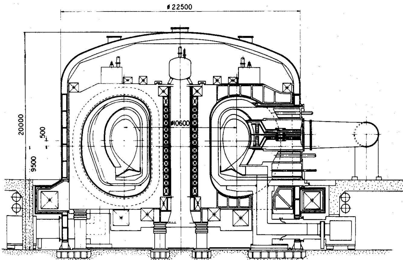
Fig. 1. Elevation view of INTOR phase IIA configuration.
