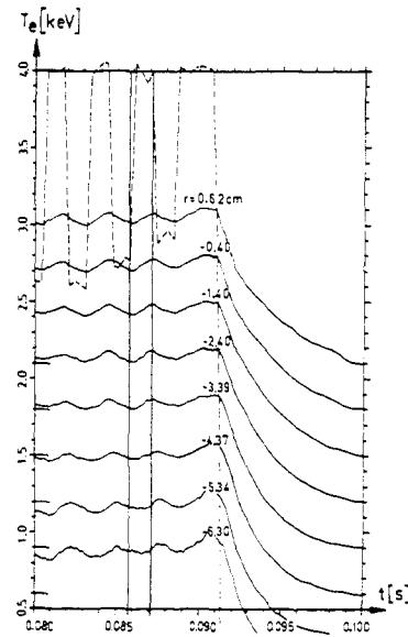
Fig. 14 Time variation of ECE measured electron temperature for different plasma radii.
