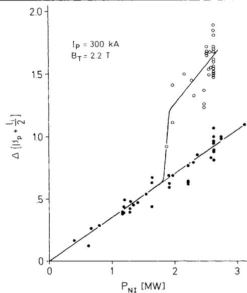
FIG. 3. Increase in  $\beta_p + \frac{1}{2} I_t$  with respect to the Ohmic phase vs the power  $P_{NI}$  injected into the vessel in the L regime (solid symbols) and the H regime (open symbols).
