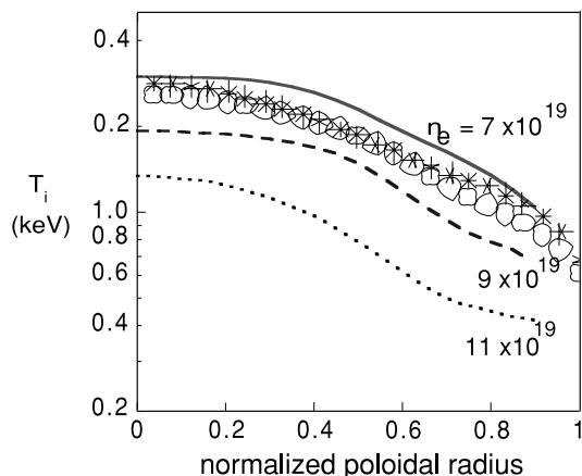
Fig. 5. H-mode ion temperature profiles measured during a density scan (lines) and for on- and off-axis heat deposition (symbols) are stiff with a constant temperature gradient length  $T/\Delta T$  in the confinement region between 0.3 and 0.8 of normalized poloidal radius.
