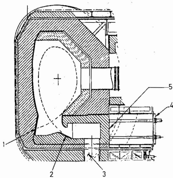
Fig. 2. INTOR divertor configuration (reference design).
