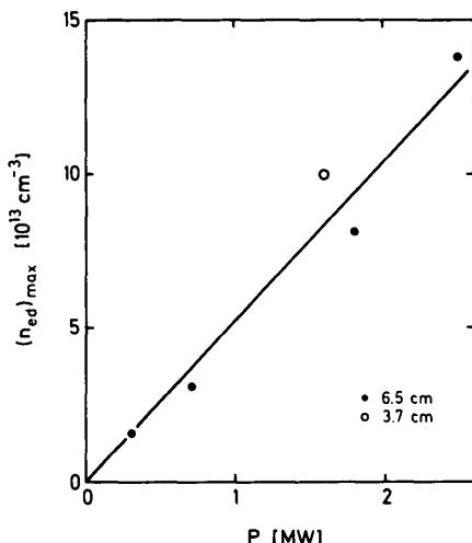
FIG. 9. Observed maximum electron density near the divertor plate  $(n_{ed})_{\text{max}}$ , as function of the heating power  $P = P_{\text{OH}} + P_{\text{NI}}$  for a divertor slit width of 6.5 cm (●) and 3.7 cm (○), respectively.
