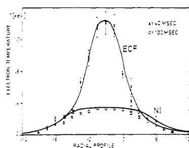
Fig. 9 A target plasma produced from the gas phase by 100 kW absorbed ECF-power is "taken over" by NBI with three injectors (220 kW absorbed power).
