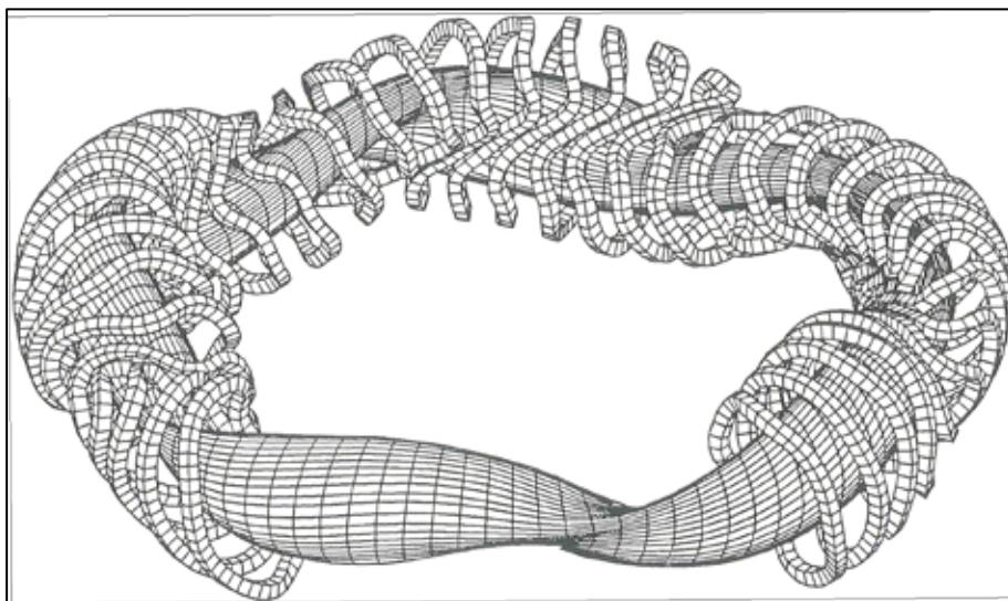
Fig. 2 Sketch of Wendelstein VII-X basic configuration. The lines on the plasma surface indicate the magnetic field lines and meridional sections, respectively.
