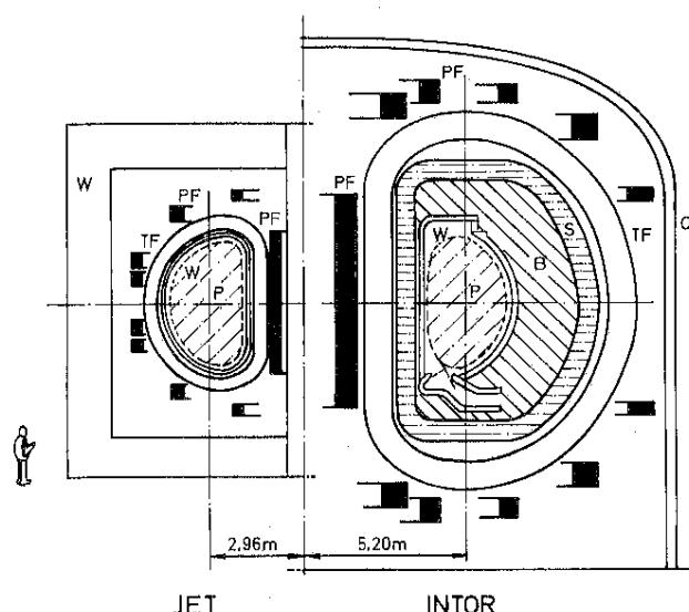
Fig. 7. In-scale comparison between JET and INTOR. Note the similar shape of the plasma cross-sections, but the difference in aspect ratio.
