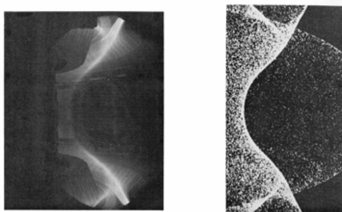
*Fig. 5 Photography of ASDEX in H<sub>α</sub>-light, illustrating the role of the divertor slits in the recycling. The picture at the right is a computer simulation based on calculated MHD equilibria clarifying the topology of the radiating zone.*
