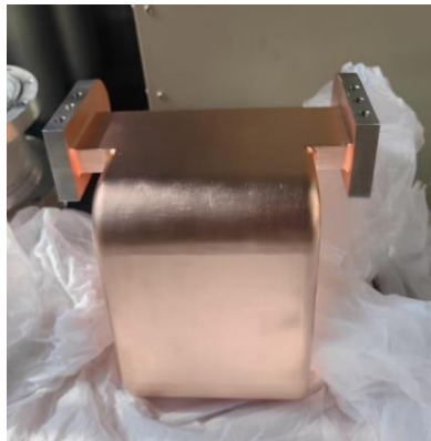
SLM strap copper coating (60 \mu m)
